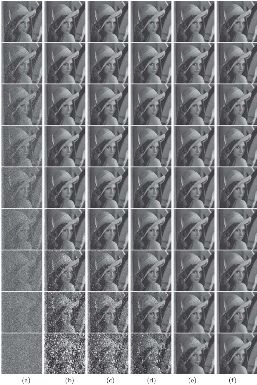
Fig. 2 Denoising output images using different algorithms (a) Salt-an-pepper noise of the lena image (10–90% noise) (b) Median filter (c) DMF (d) MCF (e) IDMF and (f) proposed method
