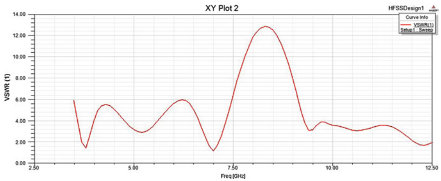
Fig. 5 VSWR plot for optimized combined T-L slot patch antenna
