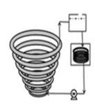
Helical tubular bioreactor
