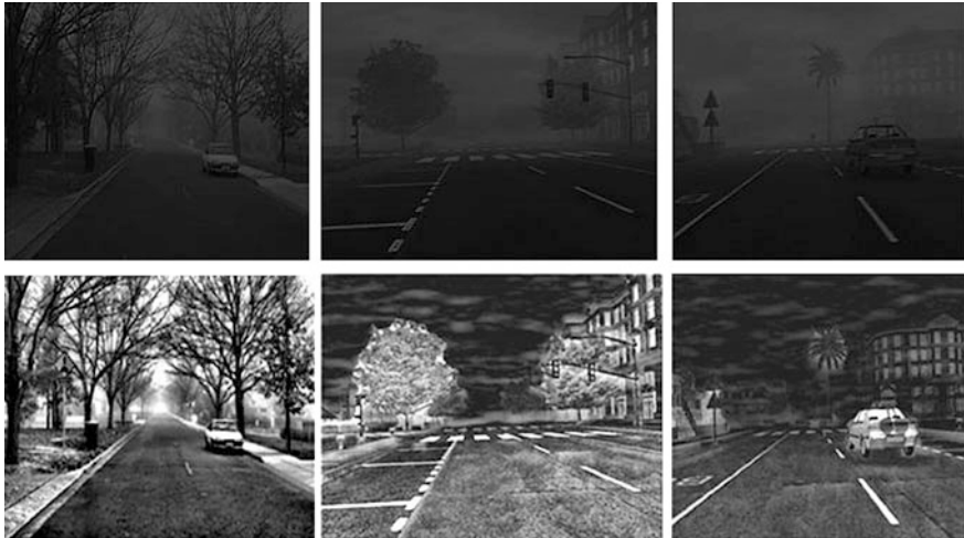
Fig. 1 Original noise images and images after used Top-hat filter
