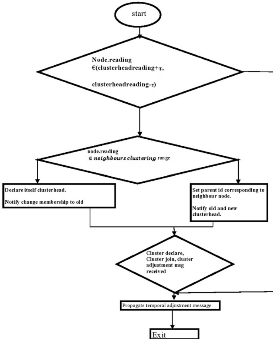
Fig. 3 Flowchart temporal adjustment timer function
