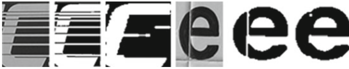
Fig. 3 Comparison of morphological operations: Original image, Average thresholding, Morphological Opening
