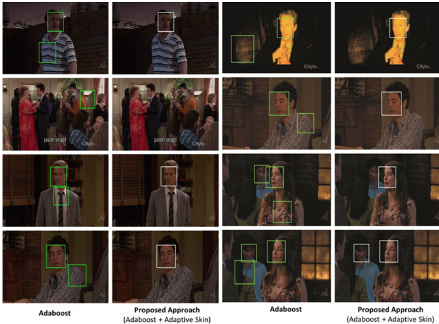
Fig. 5 Results of the proposed and Adaboost face detectors. These results are computed at T = 10 and k = 1.5
