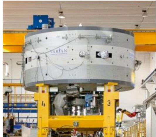
Fig. 3.12 The superconducting isochronous cyclotron from Varian Medical Systems
