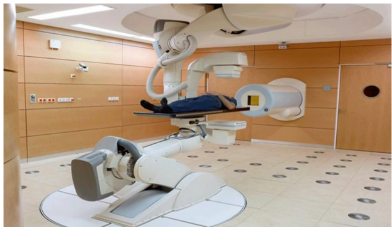
Fig. 9.10 Treatment room at the HIT facility equipped with a robotic patient positioning and imaging system
