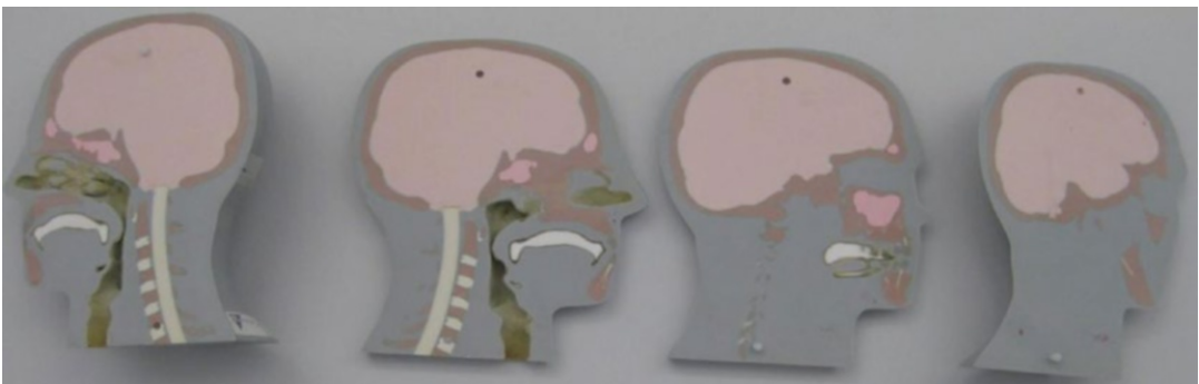
Fig. 7.16 Anthropomorphic phantom used in end-to-end tests
