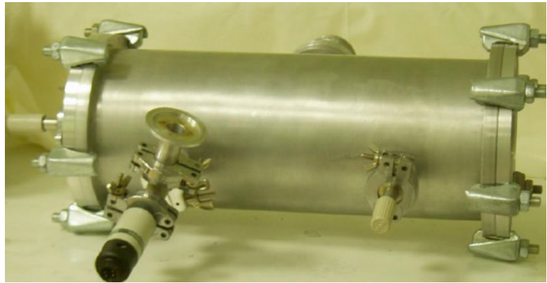
Fig. 7.12 Faraday cup (Courtesy of E. Grussel)
