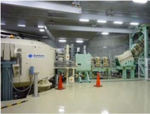
Fig. 3.11 The SHI 230 MeV isochronous cyclotron for proton therapy
