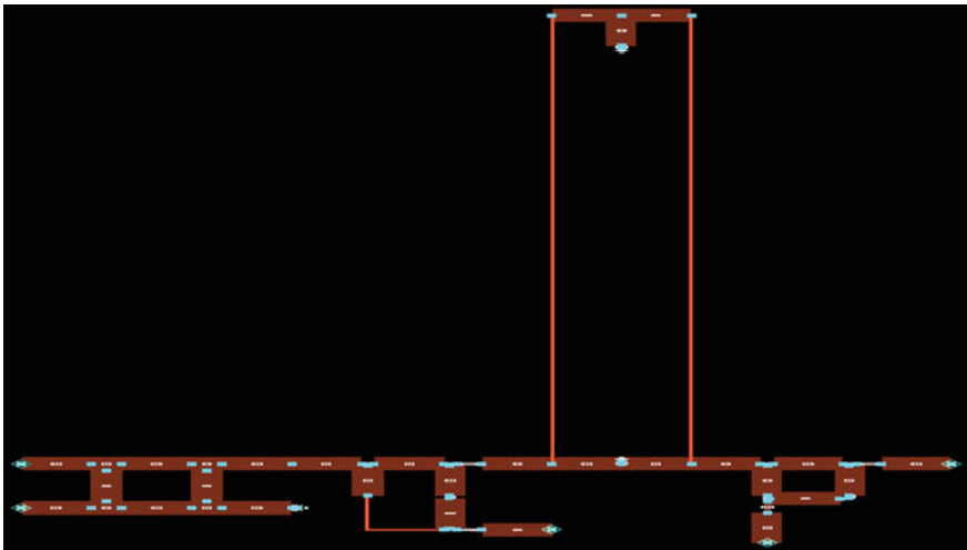
Fig. 11 Layout of the five port structure design
