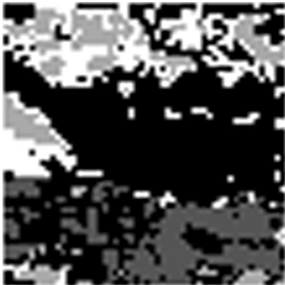
Fig. 4 Pixel classification of Ajoy River catchment area (partial) obtained FCM algorithm (with K = 7 )
