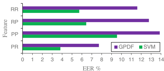
Fig. 3 Performance comparison of four keystroke features without fusion
