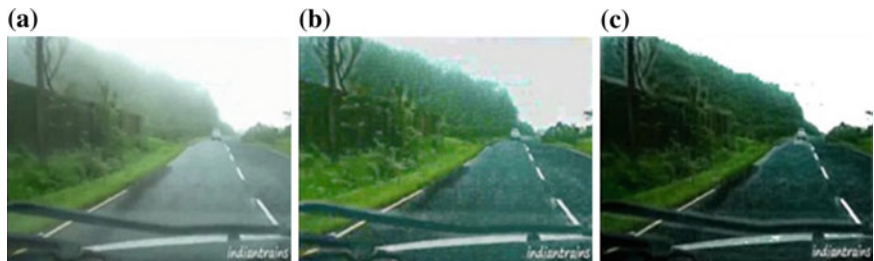
Fig. 9 a Original hazyimage b Dehazing by Tarel et al. c Proposed method output
