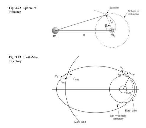
Consider two bodies and satellite as shown in Fig. 3.22. The sphere of influence or activity sphere of  $m_2$  is defined by
