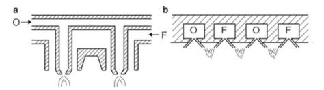
Fig. 9.24 Types of injectors (a) Co-axial (b) Doublet
