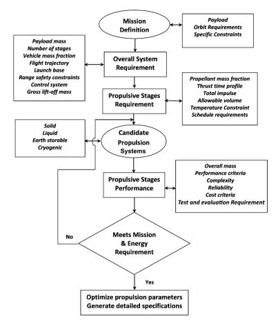
Fig. 9.2 Typical selection methodology for a propulsion system
