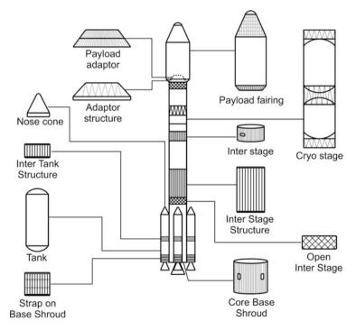
Fig. 11.1 Structures used in a typical STS
