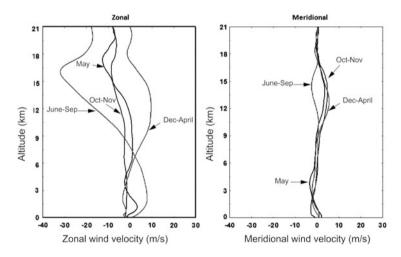
Fig. 6.25 Mean wind at a typical launch site
