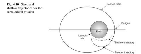
geo-transfer orbit (GTO) mission, the vehicle has to target the injection of the satellite at the perigee, which is the lowest point on the orbit. This ensures the maximum possible shallow trajectory for the mission, increasing the payload carrying capability of STS.
