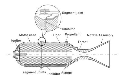
Fig. 9.16 A typical solid motor
