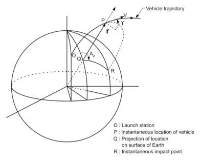
Fig. 7.31 Instantaneous impact point (stage impact)
