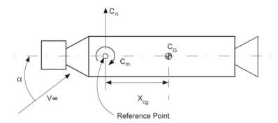
Fig. 10.37 Free molecular flight regime aerodynamic configuration
