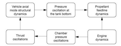
Fig. 6.35 Vehicle systems interactions in POGO phenomenon
