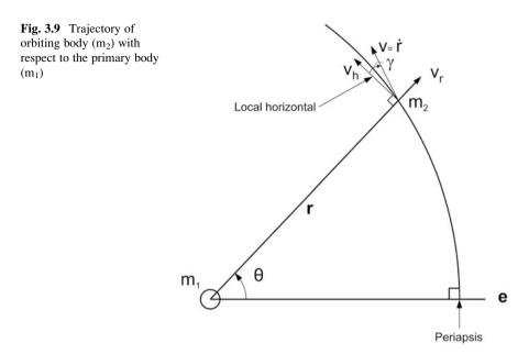
apoapsis are referred to as perigee and apogee, respectively. For the case of motion about the Sun, the corresponding points are called perihelion and aphelion, respectively. Typical trajectory of a smaller body  $m_2$  about the bigger body  $m_1$  is represented in Fig. 3.9.
