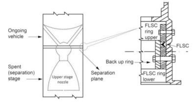
Fig. 13.21 A typical FLSC based separation system
