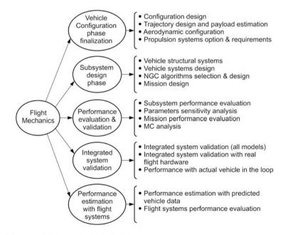
Fig. 8.1 Role of flight mechanics in STS design
