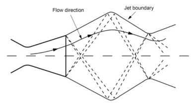
Fig. 9.9 Under expansion flow pattern
