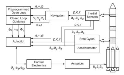
Fig. 14.2 Functional configuration of NGC system
