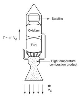
produced is  $\dot{m}V_e$ . As per Newton's third law, the thrust force acting on the vehicle is given by
