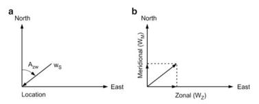
Fig. 6.11 Wind representations (a) Speed and azimuth (b) Zonal - meridional component
