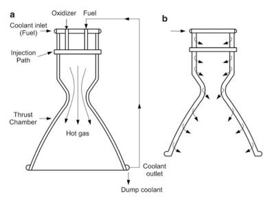
Fig. 9.25 A typical active cooling (a) Regenerative cooling (b) Film cooling
