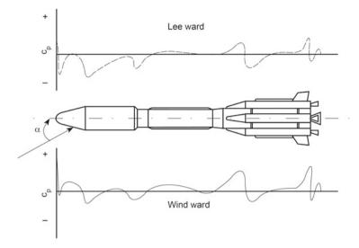
Fig. 10.21 Windward and leeward Cp distribution along vehicle length
