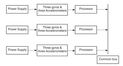
Fig. 14.12 Triple modular redundancy INS
