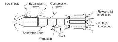
Fig. 12.8 Flow field over a vehicle
