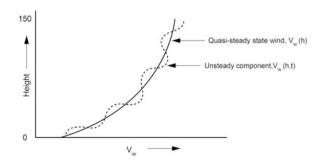
Fig. 6.21 Typical ground wind
