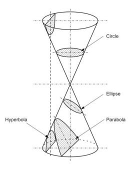
$e_c = 1$ , conic is parabola  $e_c > 1$ , conic is hyperbola
