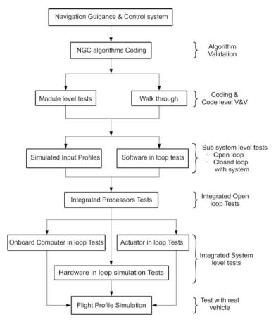
Fig. 14.37 Systematic validation procedure using various test beds
