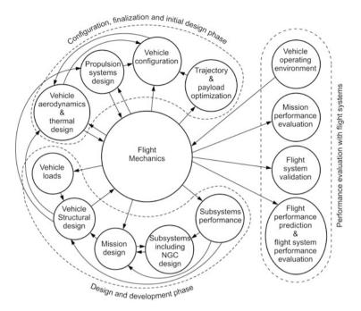
Fig. 8.2 Interactions of flight mechanics with vehicle subsystems
