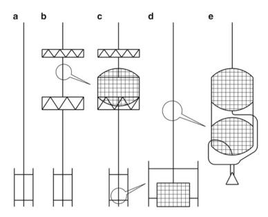
**Fig. 11.20** Typical FEM models for dynamic analysis. (**a**) Total beam model (**b**) Beam interstage model (**c**) Beam + interstage propellant tank shell model (**d**) Beam + detailed model for base shroud (**e**) Propulsion stage model
