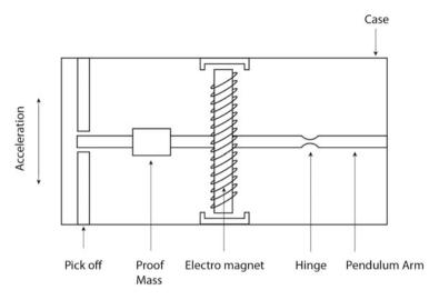
Fig. B.5 Force feedback pendulum accelerometer
