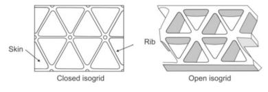
Fig. 11.10 Isogrid constructions
