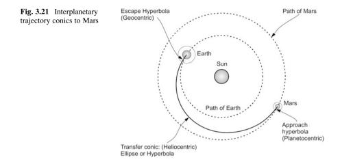
Consider an interplanetary mission from Earth to a target planet (say, Mars) as shown in Fig. 3.21. Initially, heliocentric conic section from Earth to target planet locations meeting the energy requirements and travel duration is finalized. After finalizing the requirements, the interplanetary trajectory is divided into three Keplerian conic sections as given below:
