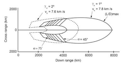
Fig. 15.20 Typical reentry foot-print
