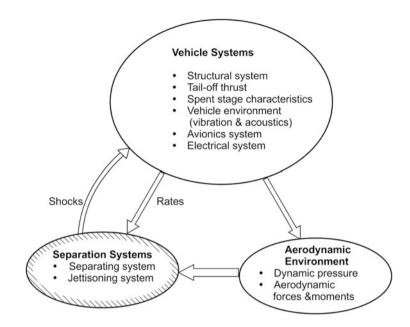
Fig. 13.3 Interaction between separation and vehicle/environment
