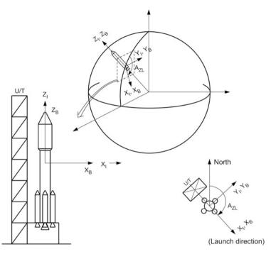
**Fig. 14.9** LPI and body frame at time = 0
