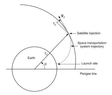
**Fig. 4.3** Satellite injection conditions and orbit  $(r_0, V_0, \gamma_0)$
