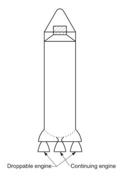
multiple small engines (Fig. 5.7b) are used. However, in both the cases, to contain large amounts of propellants, vehicle has to be configured with large tanks wherein the length and diameter of the tanks are limited by the fabrication facilities and infrastructure available. To overcome these difficulties, the staging options as explained below are to be adopted.
