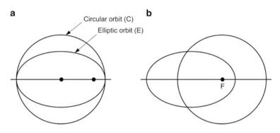
Fig. 3.11 Elliptic and circular orbits with same energy and period: (a) orbits comparison with center aligned (b) orbits about the focus
