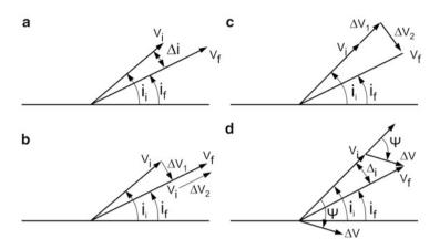
Fig. 3.29 Optimum correction for orbit size and inclination: (a) requirement (b) velocity change + Inclination change (c) inclination change + velocity change (d) inclination and orbits size change together
