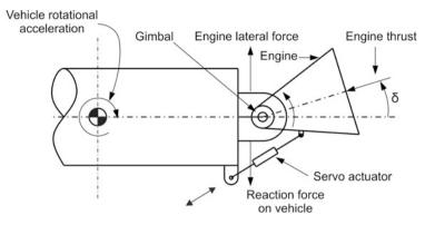
Fig. 14.28 Forces during engine gimbaling
