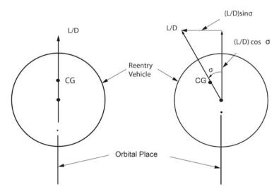
**Fig. 15.18** Bank angle  $(\sigma)$  of reentry vehicle
