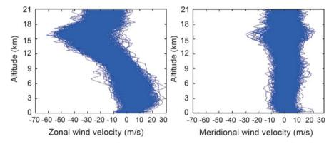
Fig. 6.23 Ensemble of measured winds over a typical launch site in a typical season
