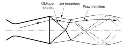
Fig. 9.11 Over expansion flow pattern
