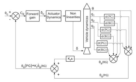
Fig. 14.25 Block Diagram for flexible vehicle system
