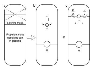
Fig. 6.33 Propellant sloshing phenomena (a) Propellant in tank (b) Pendulum mass model (c) Spring mass model
