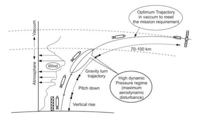
Fig. 7.4 Typical trajectory phases of an STS mission
