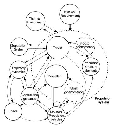
Fig. 9.1 Propulsion systems interfaces with vehicle subsystems
