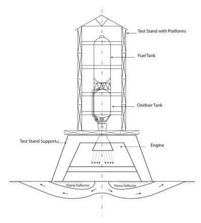
Fig. 9.31 A typical liquid stage test set up
