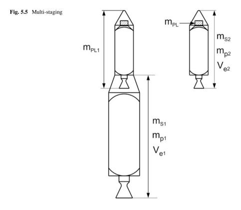
Since all stages have the same mass ratio and  $V_e$ , therefore,  $\Delta V$  imparted by each stage is given by
