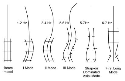
Fig. 11.21 Mode shapes of a typical vehicle
