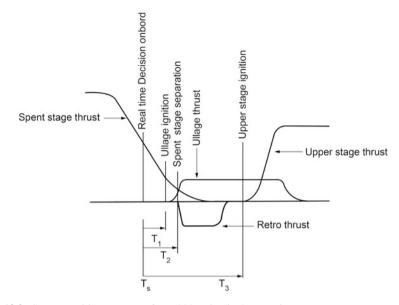
Fig. 13.9 Stage transition sequence for cold longitudinal separation process
