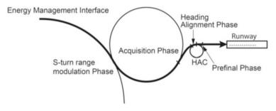
Fig. 15.40 Lateral flight trajectory of TEAM phase
