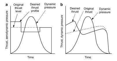
Fig. 7.8 Booster phase thrust shaping (a) Liquid engines (b) Solid motors
