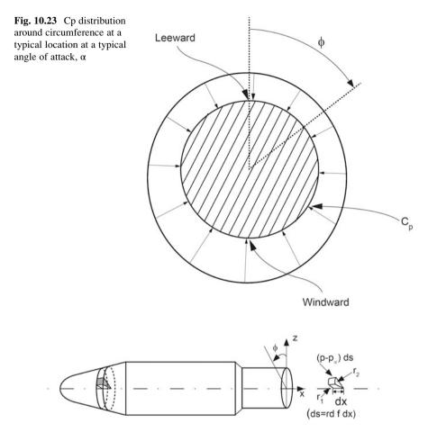
Fig. 10.24 Infinitesimal element and aerodynamic force due to pressure distribution
