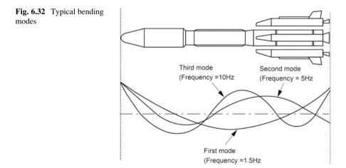
flexible modes play a major role in the dynamic environment to the vehicle systems as well as vehicle systems design. Details are given in chapters on vehicle structural systems and NGC systems design.
