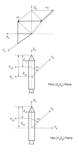
The atmospheric relative velocity of the vehicle with respect to ECI frame,  $V_{AI}$  is expressed in body frame as
