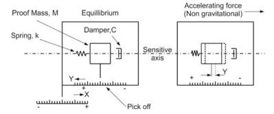
Fig. B.4 Principles of a simple accelerometer
