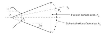
Fig. 9.7 Conical nozzle configuration
