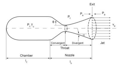
Fig. 9.4 A typical nozzle cross section
