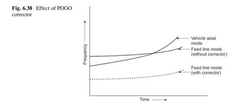
frequency. However, the propulsion system frequency can be altered by adding gas-filled cavities to the feed lines.
