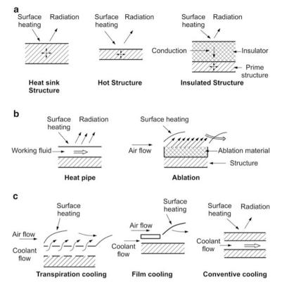
Fig. 12.5 Types of TPS (a) Passive TPS, (b) Semi-Passive TPS, (c) Active TPS
