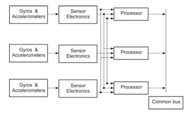
Fig. 14.13 Advanced fault tolerant architecture
