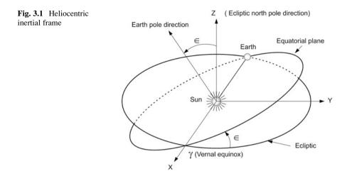
and completes the right-handed system as given in Fig. 3.1. Even though the Vernal equinox is not fixed in space, still the heliocentric reference frame is considered as an inertial frame for most of our missions since the time duration of most of the missions are much smaller than the period of variations of the reference X-axis (Vernal equinox).
