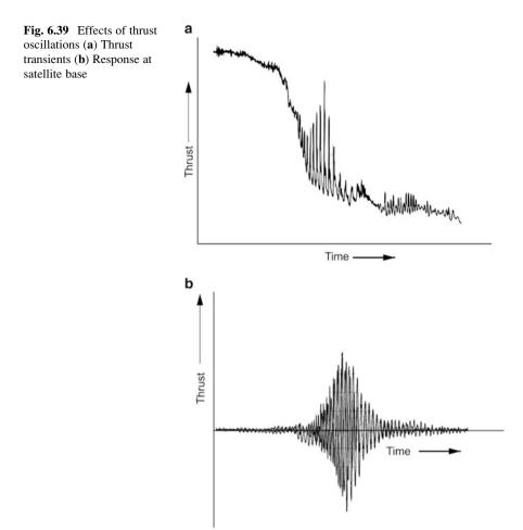
response of the vehicle due to resonance. A typical thrust transient and the corresponding dynamic loads at the satellite/space transportation system interface are represented in Fig. 6.39.
