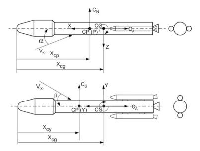
Fig. 10.11 Aerodynamic force and moment of a launch vehicle
