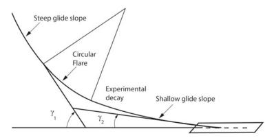
Fig. 15.41 Autolanding geometry and phases
