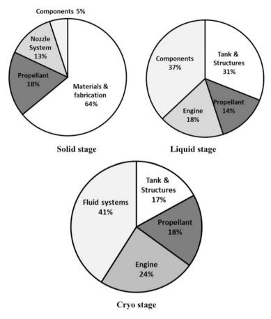
Fig. 1.3 Cost for different propulsion system
