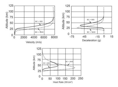
Fig. 15.10 Reentry trajectories and flight parameters for ballistic bodies with different ballistic coefficients for a typical flight path angle
