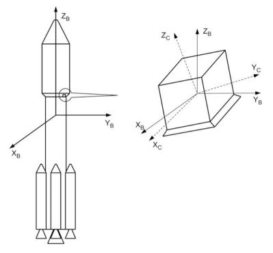
Fig. 14.8 Typical mounting configuration of sensors
