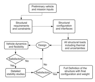
Fig. 11.4 Structures design methodology
