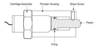
Fig. 13.25 Pyro thruster with shear screws
