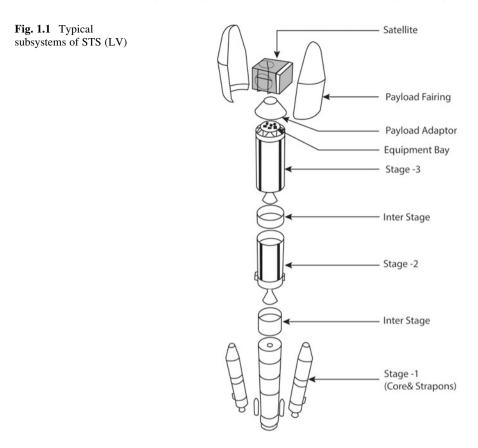
Various subsystems of a typical three stage launch vehicle are given in Fig. 1.1. The core and strap on motors form the stage-1 of propulsive elements, and stage-2 and stage-3 are other propulsion systems. Structural subsystems are the hardware of propulsive systems, inter-stages, payload fairing, payload adaptor and the structural element of equipment bay. Vehicle navigation, guidance and control systems and other avionics systems are accommodated in the equipment bay.
