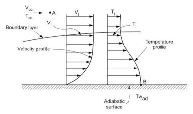
Fig. 12.1 Velocity and temperature profile within the boundary layer
