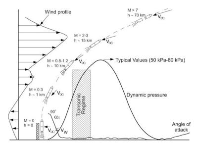
Fig. 10.7 Flight environment during atmospheric phase of a launch vehicle
