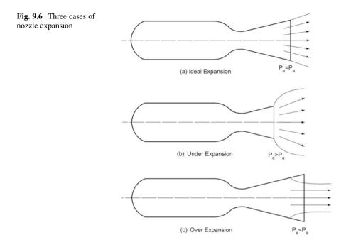
pressure thrust becomes negative. Therefore, even though there is increase in momentum thrust, the net thrust reduces. Maximum thrust occurs when there is no pressure thrust, i.e. when  $P_e = P_a$ . In an ideal nozzle the pressure of the exhaust gas at nozzle exit should be equal to atmospheric pressure, i.e.  $P_e = P_a$ . In such cases the nozzle expansion is to the ambient.
