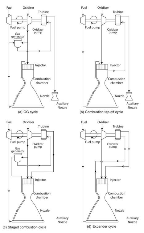
Fig. 9.20 Typical feed system cycles used in turbopumps
