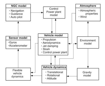
Fig. 8.13 Integrated flight mechanics model
