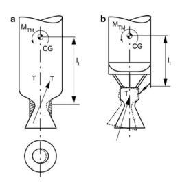
to the attachment of actuator mechanism at one side of the engine, the thrust frame deformation is non-uniform which tilts the engine at one side, as represented in Fig. 6.28b. As the thrust is along the axis of the deflected engine, this tilt causes the disturbance moment.
