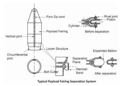
Fig. 13.30 A typical payload fairing separation system
