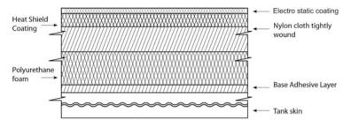
Fig. 12.19 Typical insulation system for cryo-system
