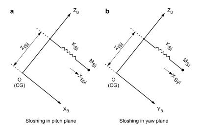
Fig. 8.11 Spring mass analogy of liquid sloshing. (a) Sloshing in pitch plane. (b) Sloshing in yaw plane
