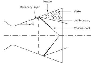
originated at the nozzle exit. This compression is followed by expansion and subsequently compression waves and so on as shown in Fig. 9.11.
