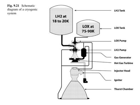
drive the propellants from tank to the thrust chamber at the rated pressure and flow rate. The pumps are driven using the hot gases generated by the gas generator or pre-burner. In GG cycle the gas generator produces the hot gas by burning the small quantity of LOX and LH<sub>2</sub> bled from outlet of respective pumps. In SCC, hot gas is generated by burning the full hydrogen after regenerative cooling of thrust chamber and small quantity of LOX bled from pump outlet.
