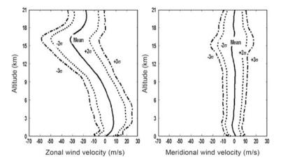
Fig. 6.24 Mean wind and dispersion band of typical season
