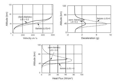
Fig. 15.14 Effect of adding lift to ballistic body on trajectory, deceleration load and heat rate
