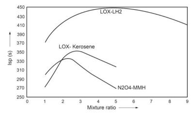
Fig. 9.15 Dependence of Isp on mixture ratio for different propellant combinations
