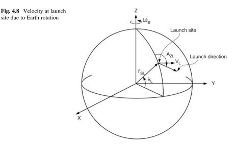
This eastward velocity,  $V_L$  at the location of launch site has the component along the launch azimuth direction as given by
