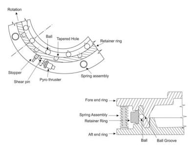
Fig. 13.24 A typical ball lock separation mechanism
