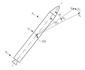
effects  $\alpha_{err}$  and  $\alpha_f$ . Therefore, the presence of shear in the wind profile introduces higher angle of attack  $\alpha$  and in turn higher aerodynamic load. Even if the absolute wind speed is less, the presence of wind shear causes larger angle of attack. As the wind shear increases, the load induced by  $\alpha_W$  also increases and finally ends up with gust response.
