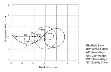
Fig. 14.29 Validation of autopilot in frequency domain
