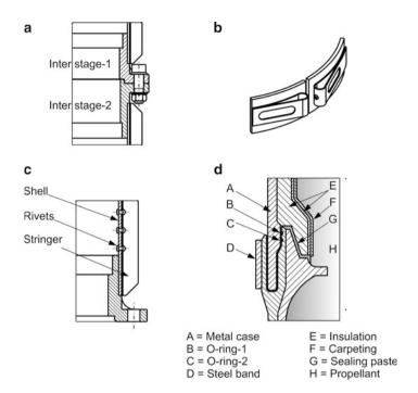
Fig. 11.6 Different types of structural joints. (a) Flanged joint (b) Merman Band joint (c) Riveted joint (d) Tongue and groove joint
