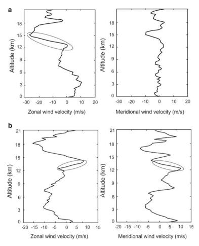
Fig. 6.17 Wind shear in typical measured wind profiles (a) Shear in magnitude (b) Diectional shear
