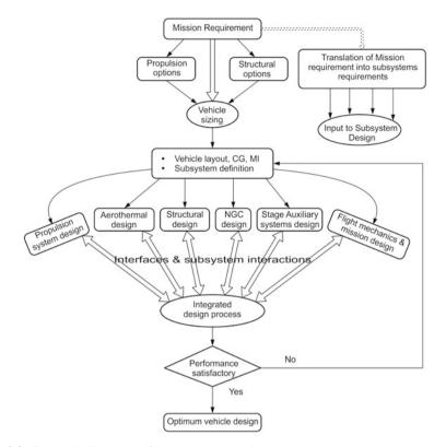
Fig. 2.3 Overall design process for space transportation system
