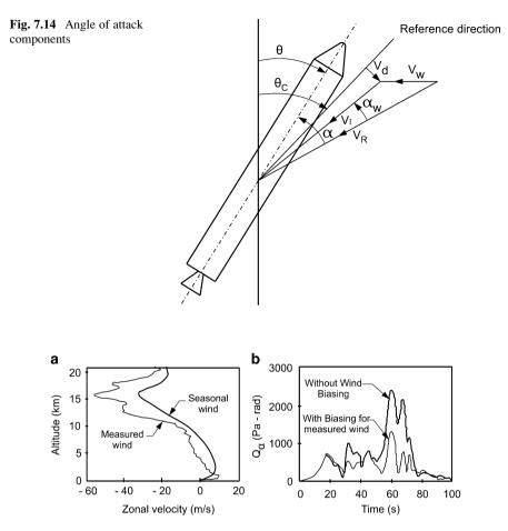
Fig. 7.15 Impact of seasonal wind biasing (a) Wind (b) Aero load indicator
