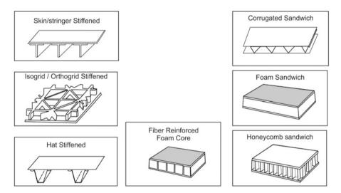
Fig. 11.11 Composite structural compositions
