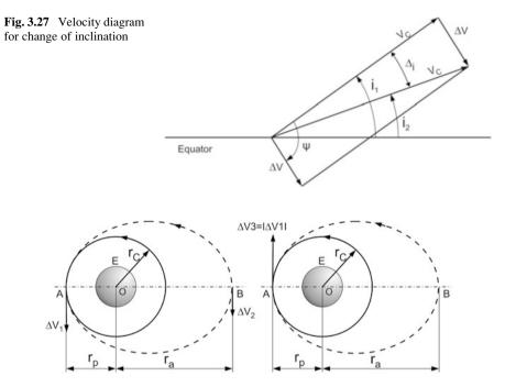
Fig. 3.28 Optimum inclination correction maneuvers
