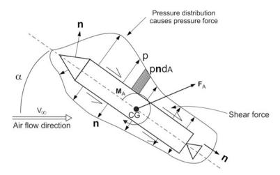
Fig. 10.8 Aerodynamic force and moment generation phenomenon
