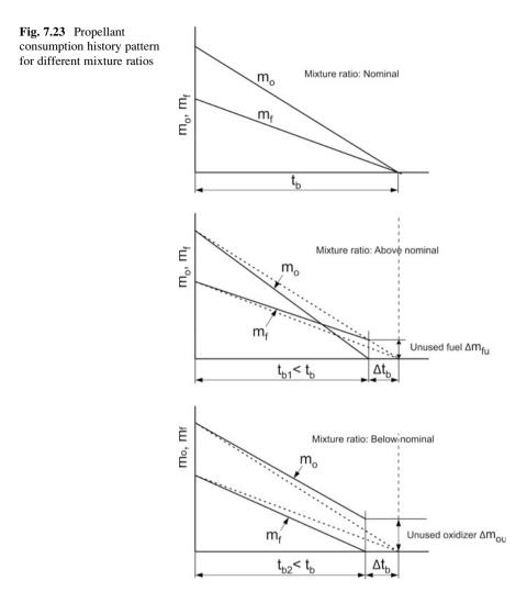
However, due to the errors in sensors used for the mixture ratio control as well as due to the deviations in the subsystems used with respect to the predicted values, there can be small dispersions in the realized mixture ratio. The deviated mixture ratio and the propellant depletion before the expected time have the following implications: (1) reduction in the active functional duration of the stage, (2) tail-off characteristics.
