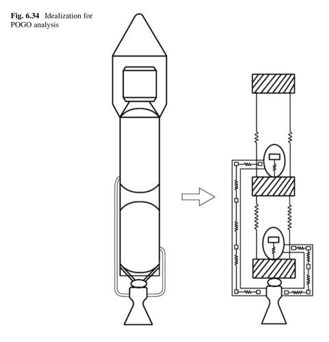
dynamics leads to POGO oscillations. In order to understand the POGO phenomenon, the POGO dynamics of the propulsion system is idealized as represented in Fig. 6.34.
