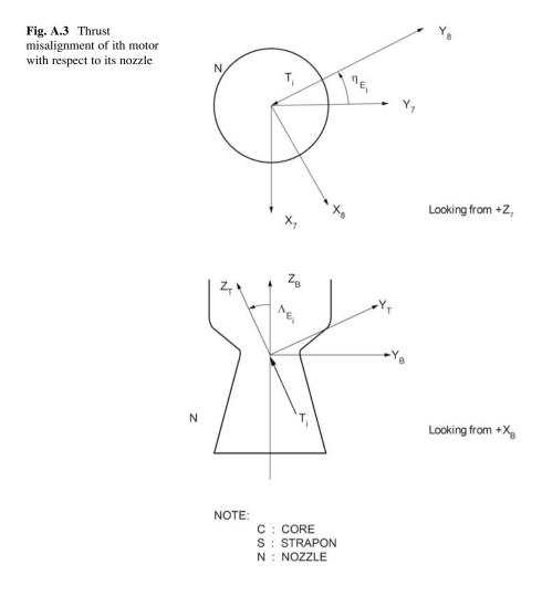
The unit vector along the thrust direction can be expressed in body frame using the transformation matrix generated from the following sequence of Euler angle rotations:
