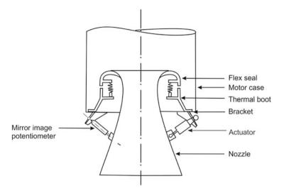
Fig. 14.34 Typical flex nozzle control system
