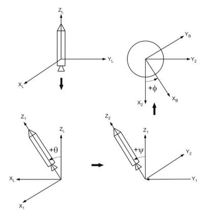
Fig. 8.7 Transformations from ECI Frame to body frame
