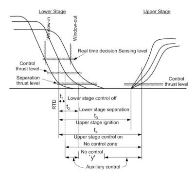
Fig. 7.22 Typical stage transition sequencing
