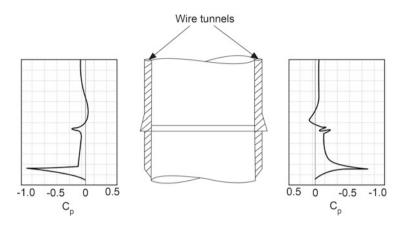
Fig. 10.32 Loads of typical wire tunnel ducts
