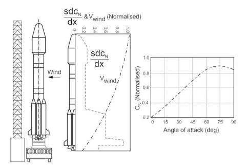
Fig. 10.14 Vehicle on launch pad and aerodynamic characteristics
