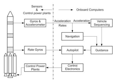
Fig. 14.1 Typical configuration of a NGC system
