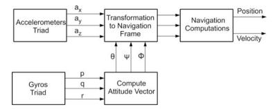
Fig. 14.5 Schematic of a strap-down navigation system
