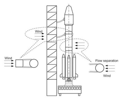
Fig. 10.13 Aerodynamicflow at launch pad
