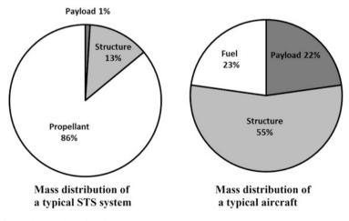
Fig. 1.5 Typical payload fractions
