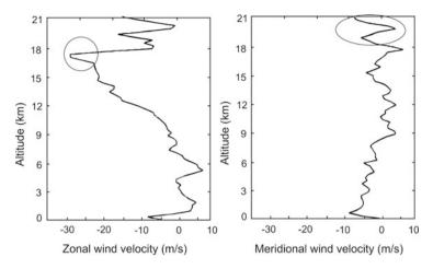
Fig. 6.18 Wind gust characteristics in a typical measured wind
