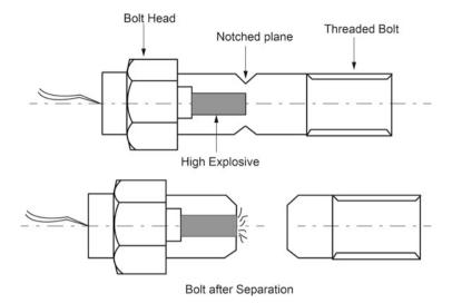
Fig. 13.18 Schematic of an explosive bolt
