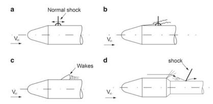
Fig. 10.26 Causes of unsteady loads. (a) Movement of shock wave during transonic regime. (b) shock boundary layer interraction cause flow separation. (c) Pressure oscillation due to wake. (d) Flow separation due to geometric shape and reattachment
