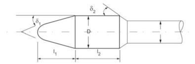
Fig. 10.27 Geometrical parameters of forebody for deciding buffet force configuration
