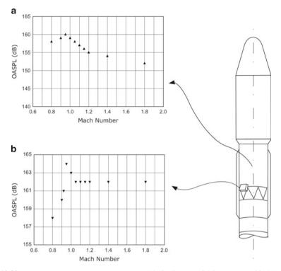
Fig. 10.30 Unsteady pressure measurement model & OASPL. (a) OASPL at a specified location (flow reattachment effect). (b) OASPL at specified locaitons (Protrusion effect)
