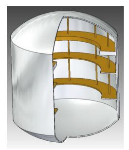
**Fig. 11.5** Baffles used in liquid tanks
