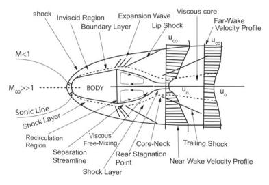
Fig. 15.22 Hypersonic flow features of a typical reentry blunt body
