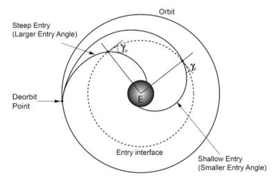
Fig. 15.12 Comparison between steeper and shallow reentry trajectories
