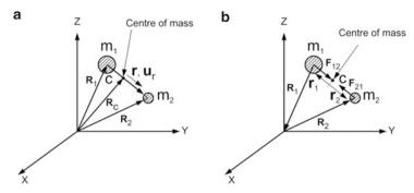
Fig. 3.4 Two-body system: (a) two bodies in inertial frame (b) free-body diagram
