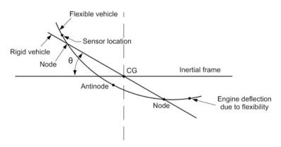
Fig. 14.27 Vehicle deflected in fundamental mode
