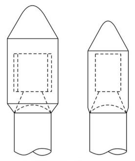
(a) Bulbous payload fairing (a) Straight payload fairing
