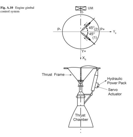
If the thrust of engine is T then the side force generated is given as
