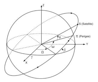
The six orbital elements corresponding to a geocentric orbit as defined in Fig. 3.14 are summarized below:
