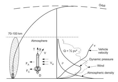
Fig. 7.7 Criticalities of atmospheric flight phase
