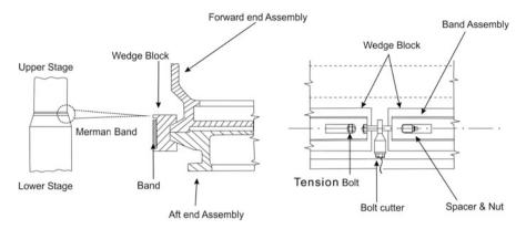
Fig. 13.22 Schematic of merman band separation system
