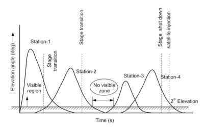
Fig. 7.30 Elevation angles of typical STS mission
