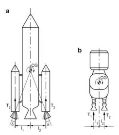
The disturbance moment due to differential thrust is minimized by utilizing the two strategies: (1) The vehicle CG is estimated at different flight instants. The nozzles of the motors are canted such that at the critical flight regime, the thrust passes through CG so that there is no disturbance moment even though there is a lateral unbalanced force. (2) Reduce the differential thrust level by adopting the pair-casting of the strap-on motors.
