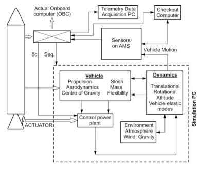
Fig. 14.39 Progressive simulation of NGC system with onboard hardware
