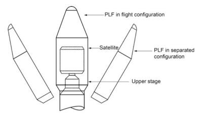
Fig. 13.13 PLF in assembled and separated configurations
