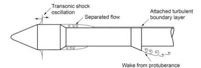
Fig. 6.40 Typical aerodynamic noise sources
