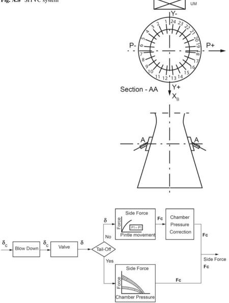
Fig. A.9 Typical modeling of SITVC system
