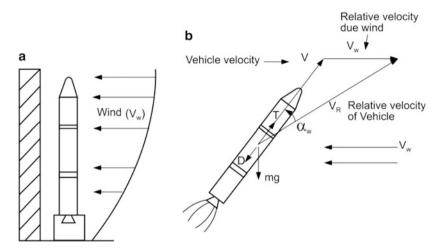
Fig. 6.12 Impact of wind on vehicle (a) Wind onvehicle atlaunch pad (b) Inflight wind on vehicle
