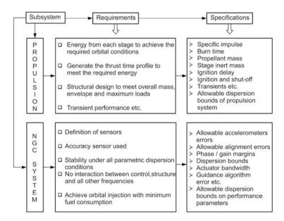
Fig. 2.5 Translation of requirements into specifications
