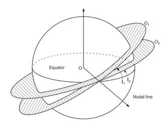
Fig. 3.26 Inclination change of circular orbits
