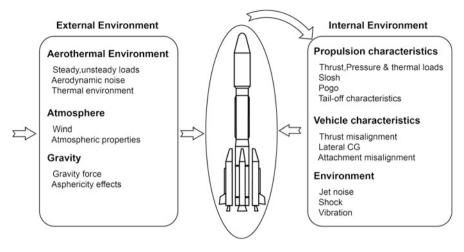
Fig. 6.1 Typical operating environments
