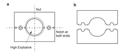
Fig. 13.19 Schematic of an explosive nut. (a) Before separation. (b) After separation
