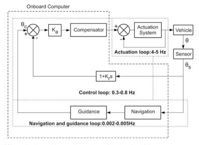
Fig. 14.20 Navigation, guidance and control loop for a launch vehicle
