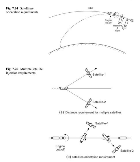
the case of inadvertent re-ignition of the separated stage, generally, the separated stage is oriented in a direction away from the satellite motion.
