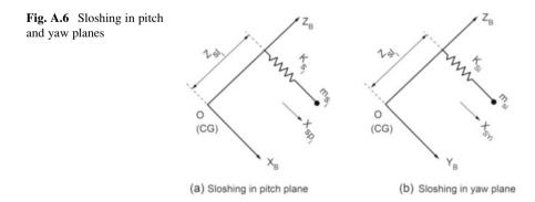
$\begin{cases} X_{s_i} \\ Y_{s_i} \\ Z_{s_i} \end{cases} = \text{Location of the ith slosh mass with respect to body reference frame} \\ \zeta_{sb_i} = \text{Viscous damping for ith slosh mass} \\ \zeta_{svert_i} = \text{Vertical baffle damping for ith slosh mass} \\ \zeta_{svert_i} = \text{Ring baffle damping for ith slosh mass} \end{cases}$
