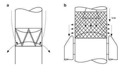
Fig. 10.35 Flowover open structures. (a) Open interstage. (b) Vented interstage
