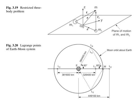
$L_1$ ,  $L_2$  and  $L_3$  are the saddle points i.e. unstable equilibrium points. The small body occupying these locations can stay there only if there is no disturbance.  $L_1$ ,  $L_2$  and  $L_3$  are the locations wherein the centrifugal force on the small mass m balances the combined collinear gravitational forces of Earth and Moon for three conditions. Due to unstable nature, any satellite placed in these points need fuel for keeping in that location.
