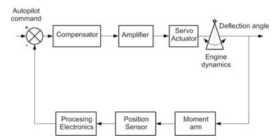
Fig. 14.30 Typical block diagram of an actuation system
