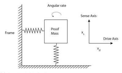
Fig. B.3 Operating principle of a vibratory gyroscope
