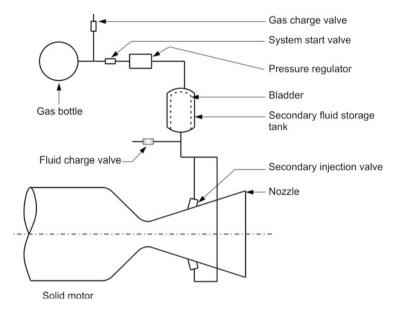
Fig. 14.32 Block diagram of a typical SITVC system
