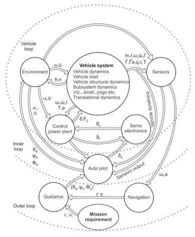
Fig. 14.3 Interactions between NGC and vehicle systems
