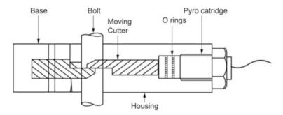
Fig. 13.17 A typical bolt cutter in action
