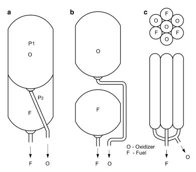
Fig. 9.23 Typical propellant tank configuration (a) Common bulkhead (b) Separate tanks (c) Multiple tanks
