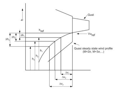
Fig. 6.26 Synthetic wind profile construction
