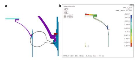
Fig. 11.13 FEM model and displacement contour of a typical pressure vessel (a) FEM model (b) Displacement
