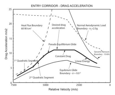
Fig. 15.35 Reentry corridor drag acceleration vs velocity
