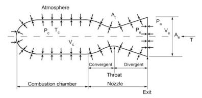
Fig. 9.3 Schematic of a rocket motor
