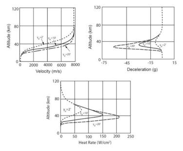
Fig. 15.11 Entry trajectories and flight parameters for various entry flight path angle for a typical ballistic body (BC = 3600)
