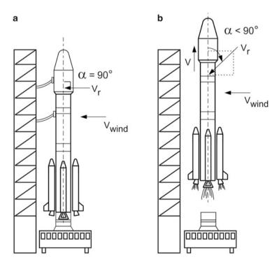
Fig. 10.12 Angle of attack during lift off phase (a) Vehicle on the Pad (b) Lift-off Phase
