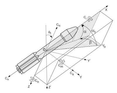
Fig. 10.9 Overall aerodynamic forces and moments on a typical launch vehicle
