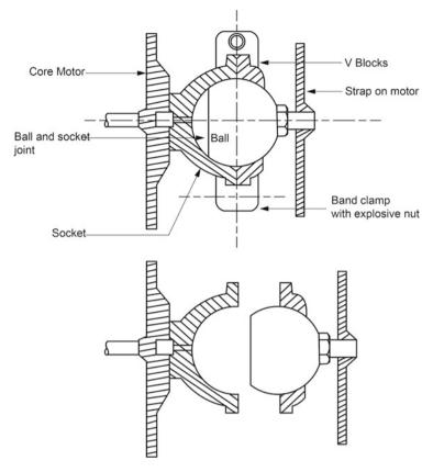
Fig. 13.29 Typical ball &socket joint
