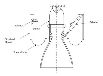
Fig. 12.18 A Typical Thermal boot used in deflectable engine
