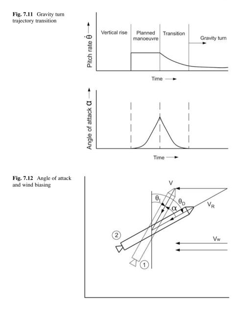
The angle of attack induces disturbing aerodynamic normal force on the vehicle. This force tends to rotate the vehicle about the centre of gravity, and the control system of the vehicle generates the necessary control force to stabilize the vehicle against the disturbances. The combined aerodynamic normal force and the balancing control force in turn introduce load on the vehicle structure. The aero-dynamic load indicator 'Qa' of a typical STS during its mission through a typical
