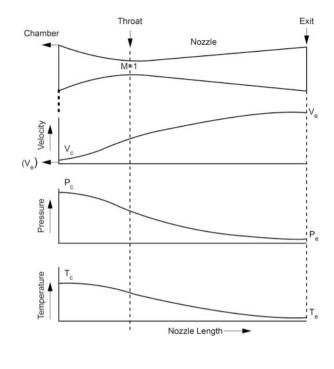
$$\frac{A_{e}}{A_{t}} = \frac{\sqrt{\gamma} [2/(\gamma+1)]^{(\gamma+1)/(2(\gamma-1))}}{\sqrt{\frac{2\gamma}{\gamma-1} \left(\frac{P_{e}}{P_{c}}\right)^{(2/\gamma)} \left[1 - \left(\frac{P_{e}}{P_{c}}\right)^{(\gamma-1)/\gamma}\right]}}$$
