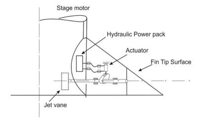
Fig. 14.31 Typical aerodynamic surface control system
