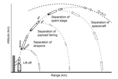
Fig. 13.1 Typical stage auxiliary systems
