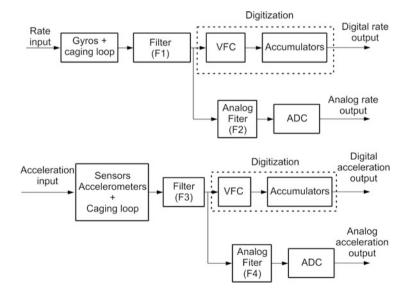
Fig. 14.6 Measurement channel of acceleration and attitude rates
