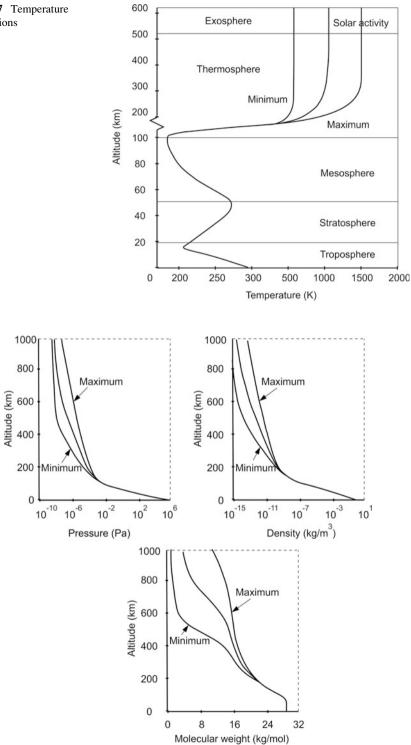
Fig. 6.8 Atmospheric properties dispersions
