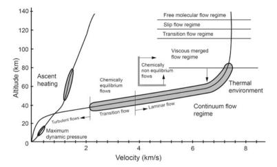
Fig. 15.2 Comparison of ascent and complex reentry flight environment
