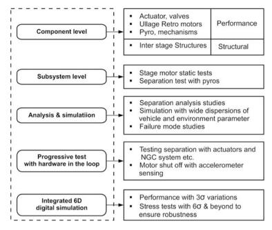
Fig. 2.8 Typical test matrix for a vehicle separation system
