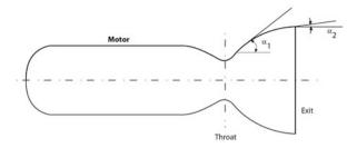
10° at nozzle exit to have uniform axial flow. For such nozzle configuration, the performance loss can be very low. Hence supersonic bell nozzle ensures better efficiency compared to straight nozzle. However, the wall contour has to be designed carefully to avoid the losses. Changing of wall contour gradually prevents the presence of oblique shocks within nozzles which have adverse impact such as flow separation and vibration.
