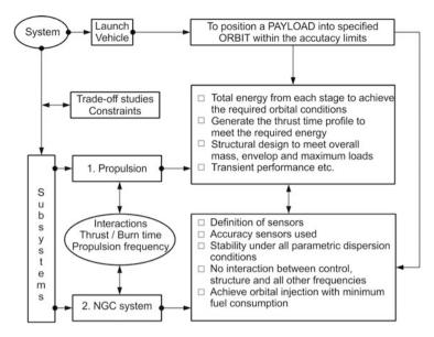
Fig. 2.4 Typical example for generation of subsystems requirements
