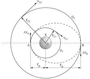
The parameters of Hohmann transfer ellipse as given in Fig. 3.24 are given below:
