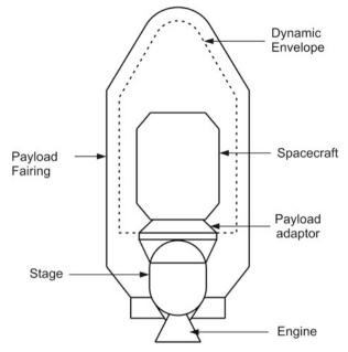
for deciding the dynamic envelope requirements. Dynamic envelope clearance has to be determined based on the detailed analysis. A typical payload envelope is as shown in Fig. 5.12.
