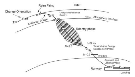
Fig. 15.27 Reentry trajectory phases of a typical winged reentry vehicle
