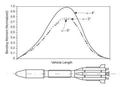
Fig. 10.28 Measured dynamic bending moment on a typical launch vehicle model
