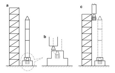
Fig. 7.6 Lateral movement during lift-off phase (a) Vehicle on pad (b) Lift-off (c) Clearing tower
