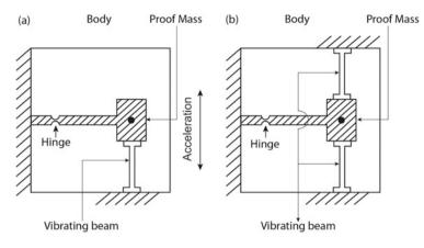
Fig. B.6 Vibratory meam accelerometer
