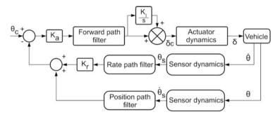
Fig. 14.21 A Typical autopilot loop
