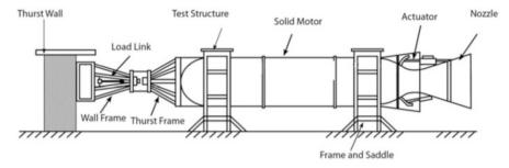
Fig. 9.30 A typical test facility for testing a solid motor
