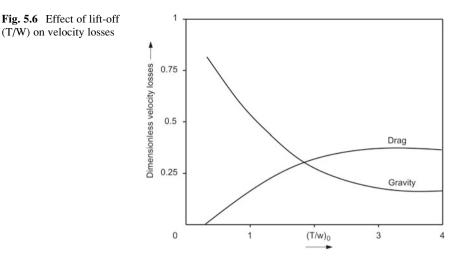
turn increases the drag loss. However, as the velocity loss due to gravity is for the entire duration of flight whereas the drag loss is only during the atmospheric flight phase, the total velocity loss during the entire mission for higher (T/W) vehicle is generally less, which in turn reduces the vehicle size. Typical dimensionless velocity losses due to gravity and drag of a typical vehicle for various levels of initial thrust-to-weight ratio (T/W) are given in Fig. 5.6.
