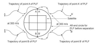
Fig. 13.14 Typical trajectory of aft end of PLF during separation process
