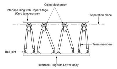
Fig. 13.26 Typical collet based separation mechanism
