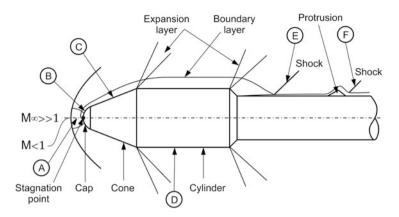
Fig. 12.9 Typical points on the payload faring
