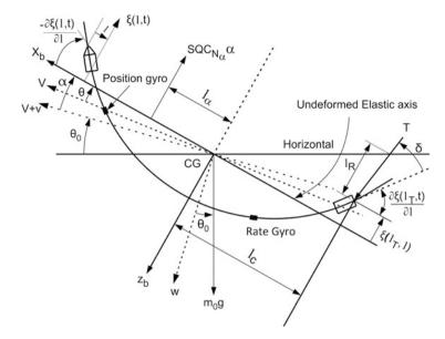
Fig. 14.24 Configuration of an elastic launch vehicle
