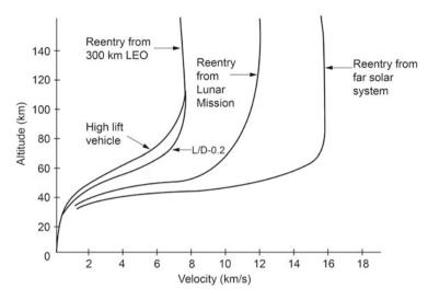
Fig. 15.3 Reentry trajectories of various return missions
