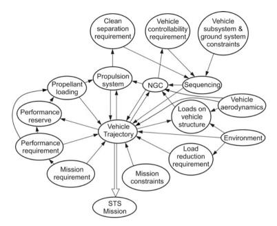
Fig. 7.2 Interactions among vehicle subsystems and mission design
