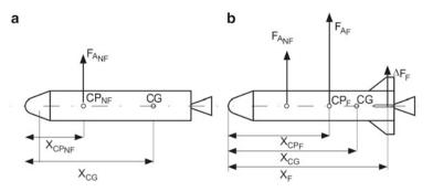
Fig. 10.42 Vehicle configuration with and without fins. (a) Vehicle without fins. (b) vehicles with fins
