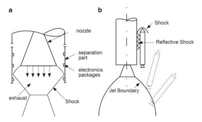
Fig. 10.36 Separation process. (a) Barrel separation. (b) Strap-on Sepration
