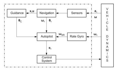
Fig. 8.12 Guidance and control system model
