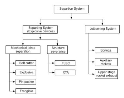
Fig. 13.2 Basic elements of a separation system
