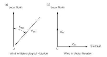
Fig. 8.10 Sign conventions for winds. (a) Wind in meteorological notatino. (b) Wind in vector notation
