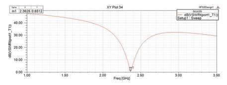
Fig. 8 VSWR curve for FSS antenna
