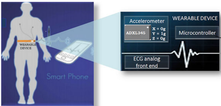
Fig. 3 Orientation of accelerometer in a wearable device
