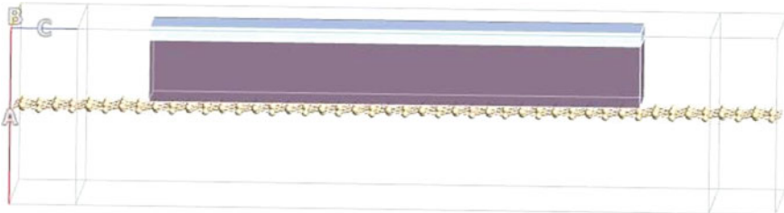
Fig. 4 FET using a channel of silicene ZNR
