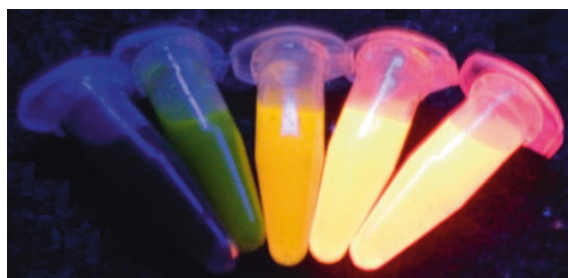
Fig. 4 Showing tuning in color of L-cysteine-capped CdTe QDs at different time intermittent fluorescence was a blinking phenomenon of QDs occurred when during crystal growth some surface defects developed in the structure act which trap the electron or hole preventing the radiative recombination and results alternation of trapping and untrapping events which cause blinking
