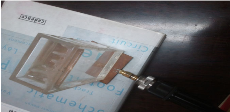
Fig. 8.13 Measurements of RDRA with aspect ratio changed
