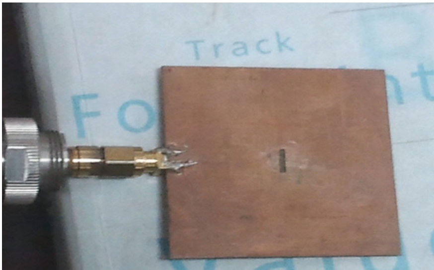
Fig. 8.16 Aperture-coupled feed showing slot
