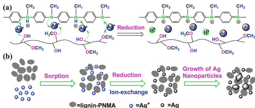
Fig. 3 Possible adsorption mechanism of \text{Ag}^+ on lignin-PNMA nanocomposites (Reprinted with permission from Lü et al. [57]. Copyright (2014), American Chemical Society)
