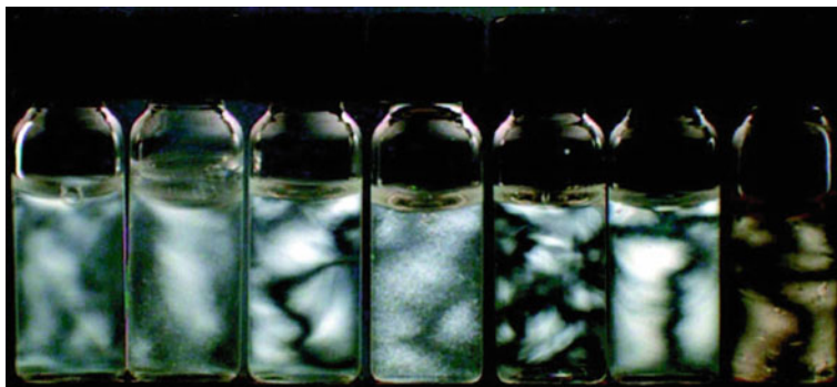
Fig. 4 Photographs of dispersions of \text{SO}_4\text{-TW} viewed through cross-polarizers at 5.0 mg/mL. From left to right as-prepared in water, freeze-dried, and re-dispersed in water, DMF, DMSO, N -methyl pyrrolidone, formic acid, and m -cresol. (Reprinted with permission from Ref. [124], Copyright © 2007, American Chemical Society)
