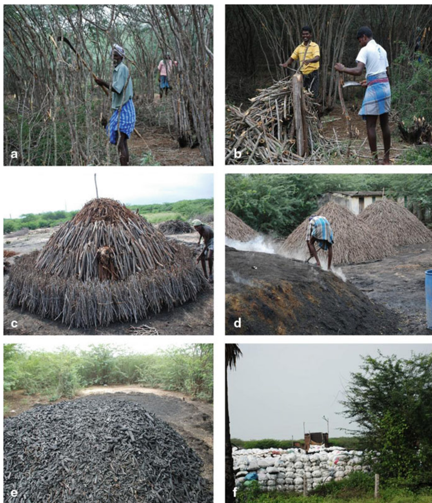
Plate 18.2 Process of charcoal production from Prosopis juliflora , a removal of secondary and tertiary branches, b cutting of wood, c and d heap making and burning, e and f charcoal produced and packed at the study sites in Ramnad district of Tamil Nadu
