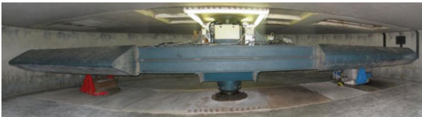
Fig. 28.17 The Cambridge 10 m diameter Turner beam centrifuge
