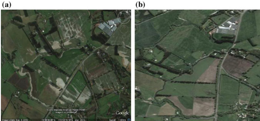
Fig. 17.6 Large liquefied site at Hoon Hay, Christchurch, New Zealand; a viewed as in Google Earth on 28 of September, 2010 by first author (Google 2010), b as viewed on Google map on 15 of December, 2012
