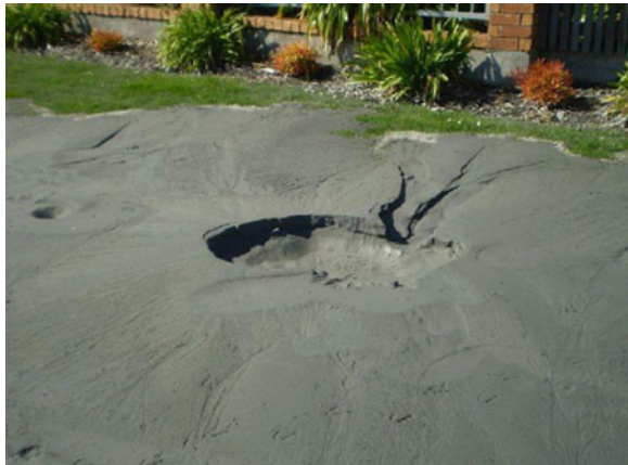
Fig. 17.4 A photo of one of the liquefaction sites that shared on Facebook on 4th of September (Rahman 2010)
