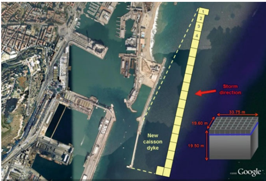
Fig. 4.1 The new caisson breakwater (background photograph Google Earth)
