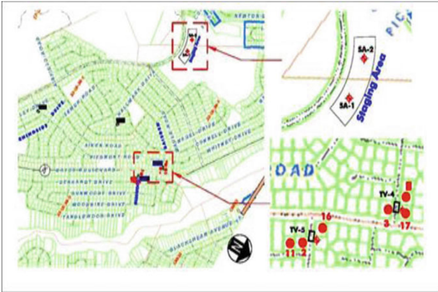
Fig. 34.6 Structure layout, with treatments vaults (TV), staging area test section (SA-1 and SA-2)
