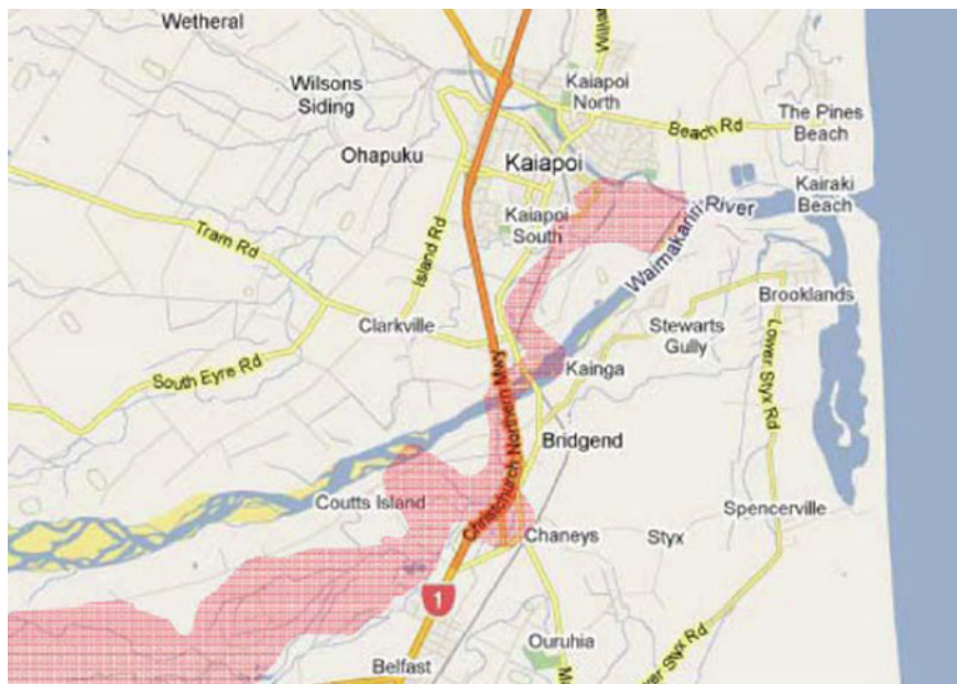
Fig. 17.1 River channel position in 1865 (in red) is presented in present day Google map (Cubrinovski et al. 2010)
