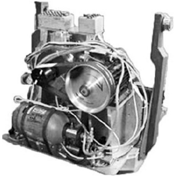
Fig. 28.18 A view of the SAM earthquake actuator
