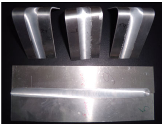
Fig. 14 Parent friction-stir welded sheet and bent samples
