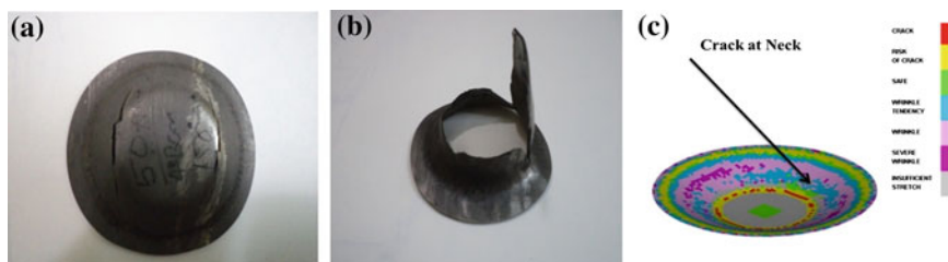
Fig. 11 Comparison of neck failure at experimentation and FE analysis using Barlat 1989 yield criterion
