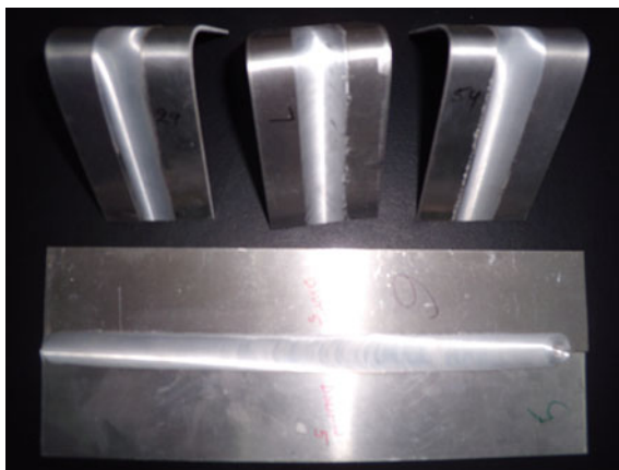
Fig. 14 Parent friction-stir welded sheet and bent samples
