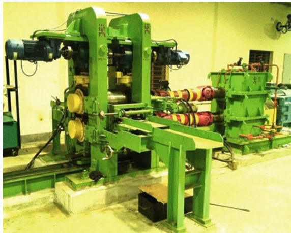
Fig. 1 2-HI rolling mill with capacity of maximum 75-ton roll separating force
