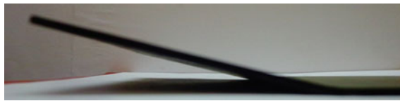
Fig. 19 Uncoated line bent specimen (power: 300 W, scan speed: 5 mm/s, number of passes: 10)
