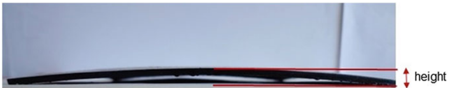
Fig. 25 Dome shaped specimen after laser forming. The horizontal red lines show the dome height measured from the base to the top most point at the center of the specimen
