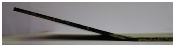
Fig. 21 Cement coated line bent specimen (power: 300 W, scan speed: 5 mm/s, number of passes: 10)
