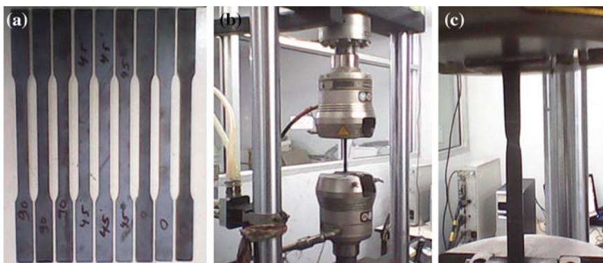
Fig. 2 Tensile test: a specimens, b setup, and c close up view of the setup
