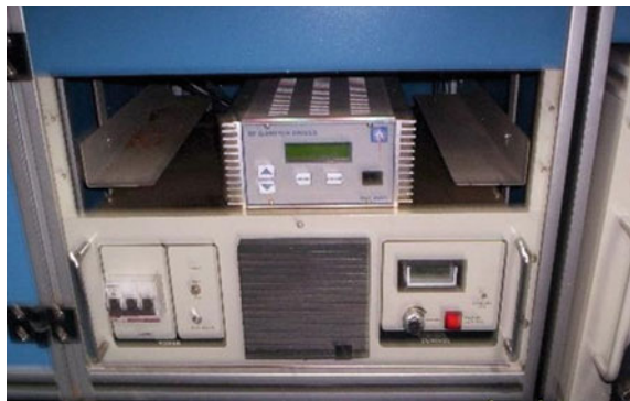
Fig. 4 The RF-Q Switch driver and the power supply (Lamp current controller) unit
