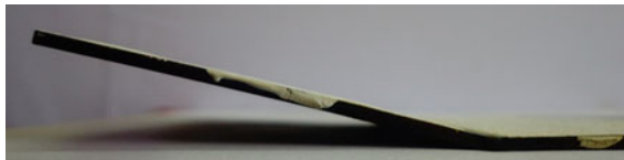
Fig. 20 Lime coated line bent specimen (power: 300 W, scan speed: 5 mm/s, number of passes: 10)
