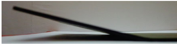
Fig. 19 Uncoated line bent specimen (power: 300 W, scan speed: 5 mm/s, number of passes: 10)
