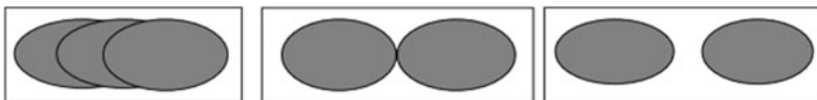
Fig. 1 Different types of spots (overlapped, continuous and discrete) formed in pulsed laser forming process
