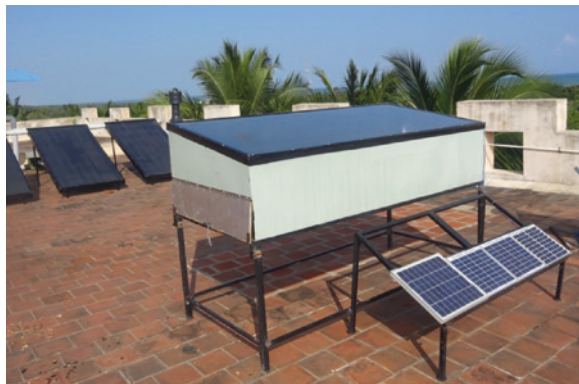
Fig. 6 Solar tunnel dryer developed at Pondicherry University
