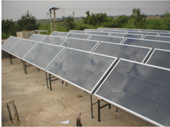
Fig. 2 Forced circulation solar air heater-based dryer developed by SPRERI
