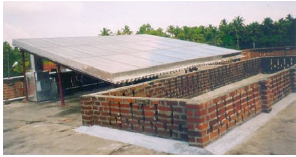
Fig. 4 Drier integrated with solar air heater—CUSAT
