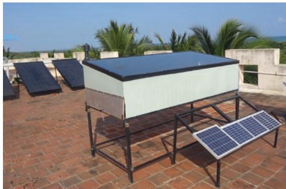
Fig. 6 Solar tunnel dryer developed at Pondicherry University
