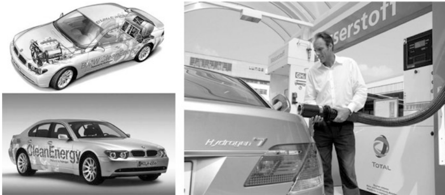
Fig. 16 One of the ICE-based hydrogen cars trialled by BMW in the past (HydrogenMotor 2007; TMR 2007)
