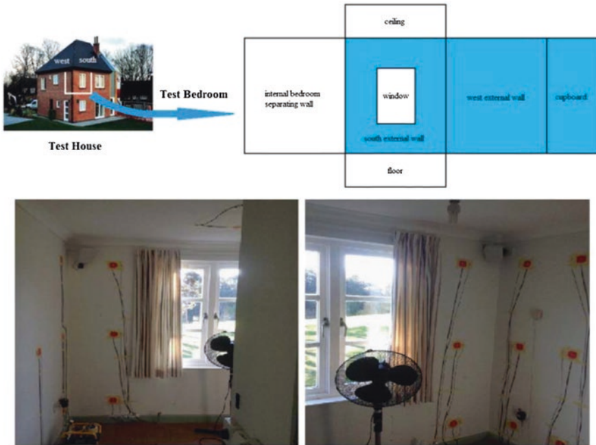
Fig. 3 Test bedroom and internal wall insulation of aerogel ( blue colored ) (Cuce et al. 2014b)
