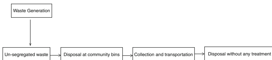
Fig. 10.1 Current waste disposal mechanism in India
