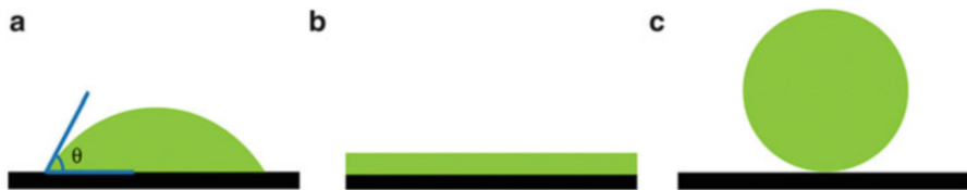
Fig. 1 A liquid drop on a flat substrate: (a) partial wetting state; (b) complete wetting state; (c) complete drying state
