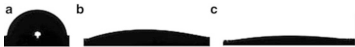
Fig. 14 Water contact angles on (a) RF sol-derived smooth carbon thin film, (b) RF sol-derived carbon nanosphere film initially, and (c) RF-derived carbon nanosphere film after 8 min (Reproduced with the permission by Sharma et al. [29])
