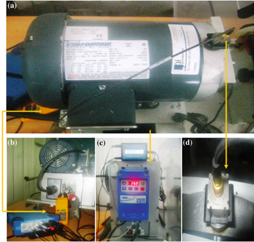
Fig. 1 Experimental setup used: a Three-phase induction motor. b Current probes and data acquisition system. c Frequency vector-based speed controller. d Triaxial industrial accelerometer
