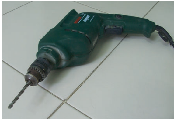
Fig. 4 Between uses, a hand-held power drill has to be kept down on its side, resting on any horizontal surface very unstably
