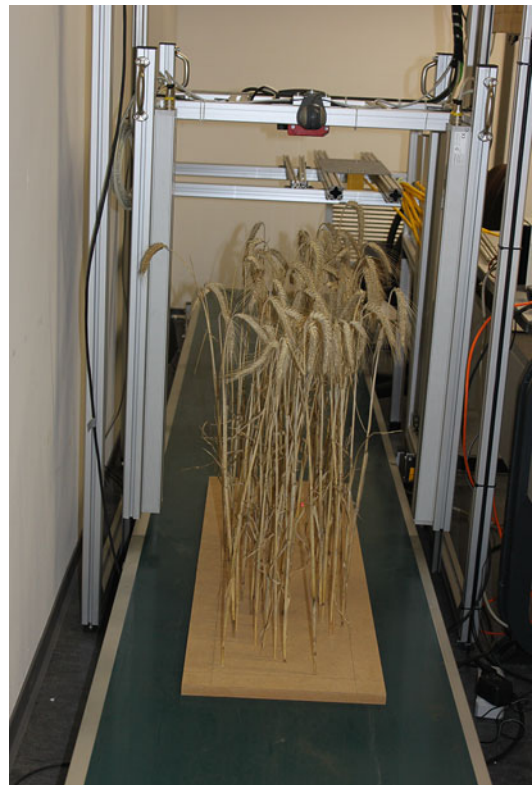
Fig. 4.2 Laboratory setup for multi-sensor phenotyping development. A conveyor belt with defined (variable) speed represents the field, while fixed sensors are evaluated with respect to their raw data and sensor fusion options in the follow-up data analysis (Photo: University of Applied Sciences, Osnabrück 2013)
