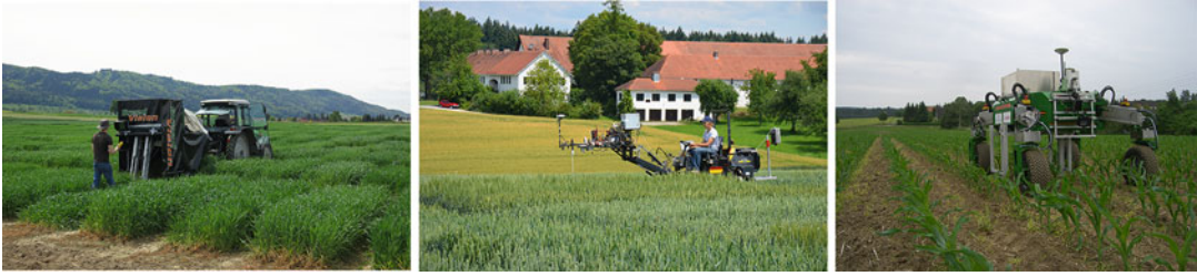
Fig. 4.3 Realized concepts of digital field-based phenotyping platforms. On the left side , the multi-sensor phenotyping BreedVision carrier is attached to a tractor (Photo: University of Applied Sciences Osnabrück, Germany 2012), the human-based special purpose vehicle
