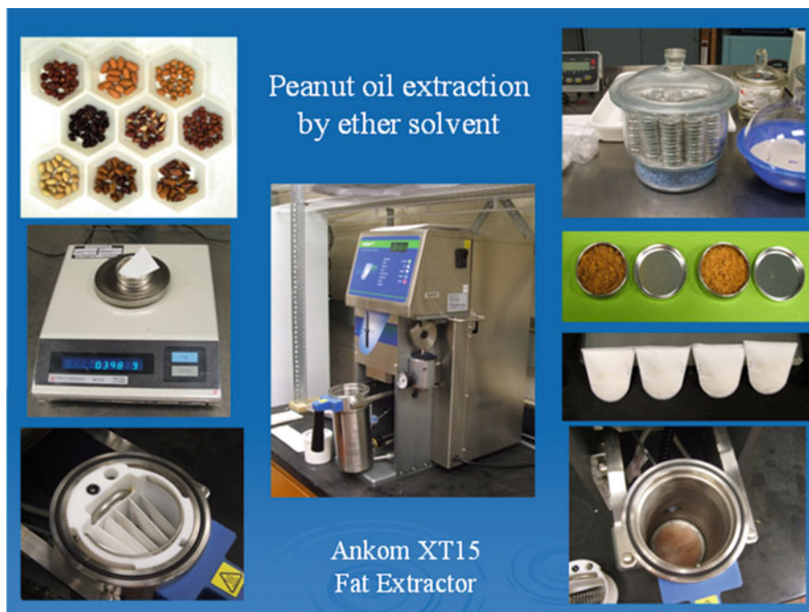
Fig. 11.4 Peanut oil extraction by ether solvent using ANKOM XT15 Fat Extractor
