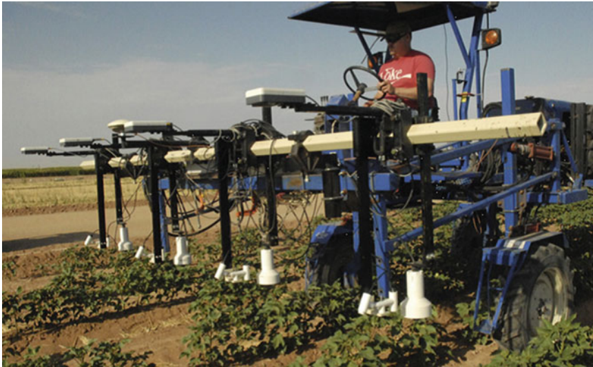
Fig. 11.2 High-clearance prototype FBP tractor in operation over young cotton plants at Maricopa, AZ, for measurement of canopy height, temperature, and spectral reflectance at three bandwidths (White et al. 2012)
