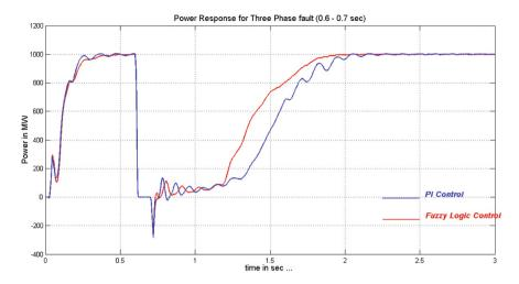
Fig. 19 Active power when a three-phase fault occurs
