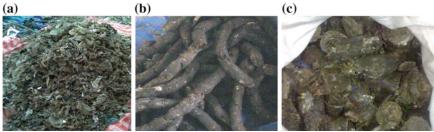
Fig. 2 a Shredded mined MSW, b Extruded mined MSW, and c RDF
