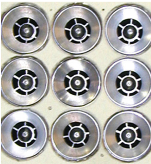
Fig. 42 The baseline 9-point SV-LDI design; from Tacina et al. (2005a)
