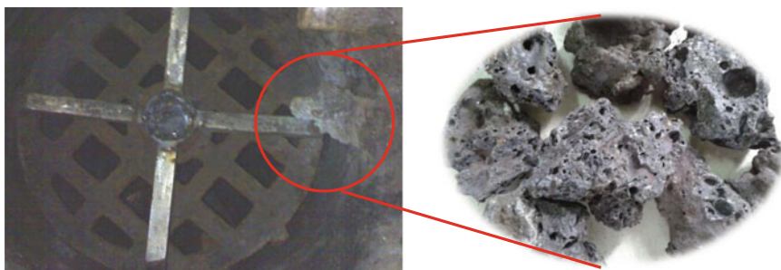
Fig. 5 Melted plastic agglomeration in the low temperature zone of gasifier
