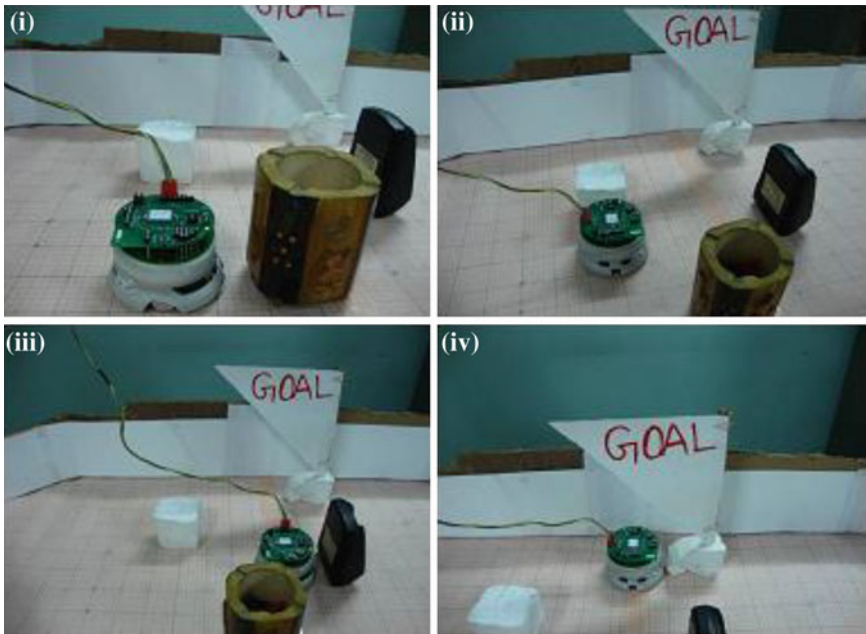
Fig. 5 Snapshots taken at different stages of path planning. (a) Initial movement of the robot to next grid. (b)–(c) Intermediate position of movement of the robot. (d) Final position of the robot at the goal
