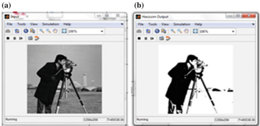
Fig. 6 Grayscale image thresholding. a Input image. b Output image
