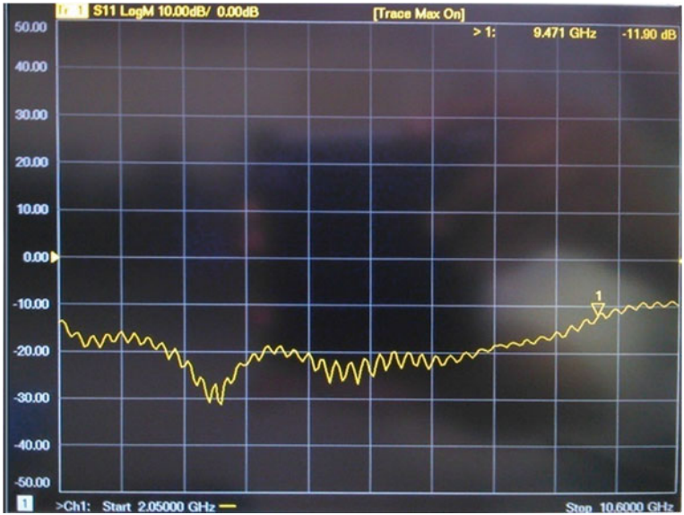
Fig. 10 Return loss plot of fabricated antenna at 5.5 GHz
