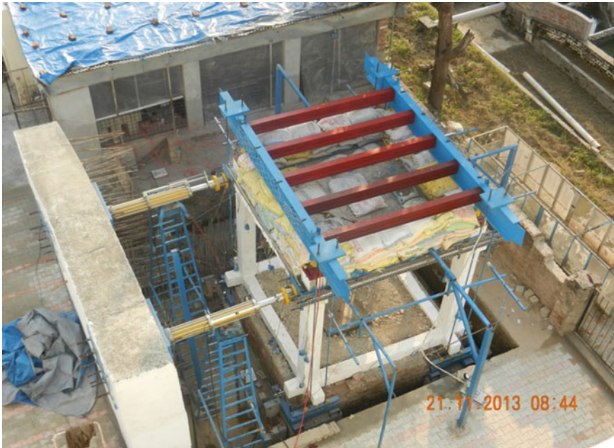
Fig. 3 Test arrangement for the seismic loading as seen from the top
