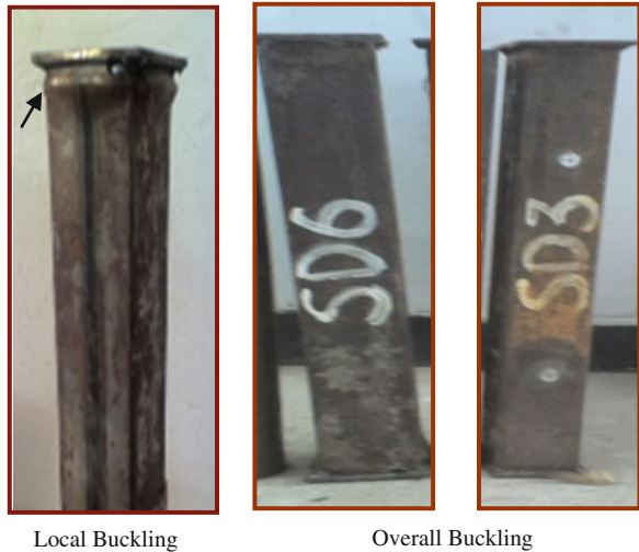
Fig. 9 Failure modes of CFT columns
