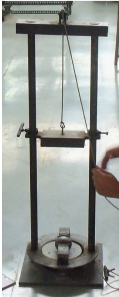
Fig. 3 Arrangement of specimen for impact test
