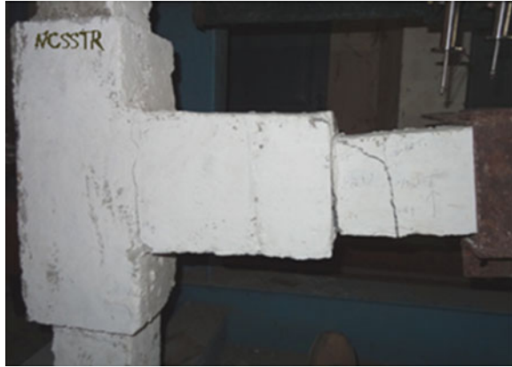
Fig. 10 Crack pattern in monolithically strengthened specimen
