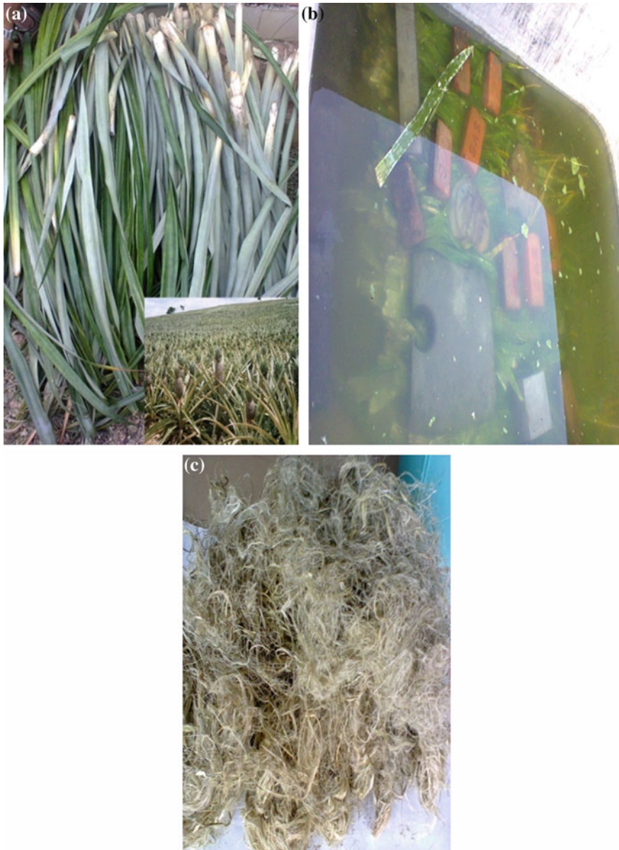
Fig. 2 a Pineapple leaves ( inset showing Pineapple fields). b Retting of Pineapple leaves. c PALF
