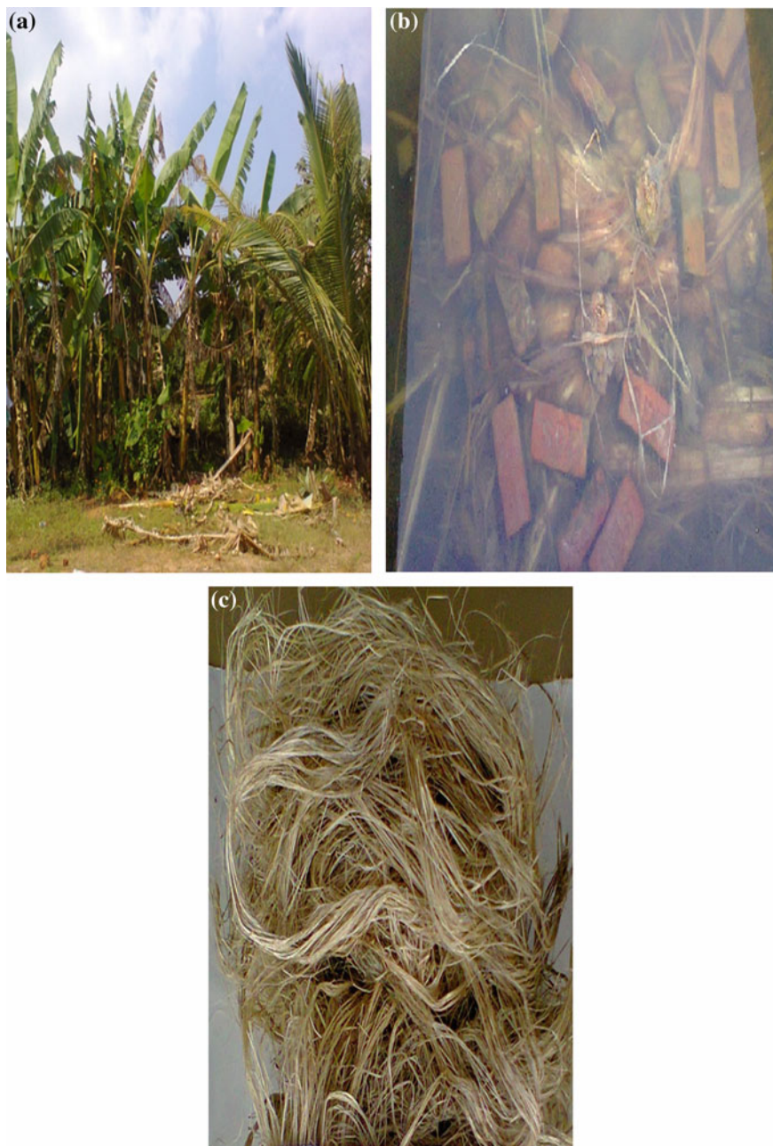
Fig. 3 a Banana plants. b Retting of Banana stems. c MUSAF
