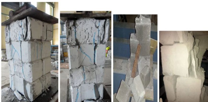
Fig. 11 Failure patterns observed in prism test for different h/t ratios
