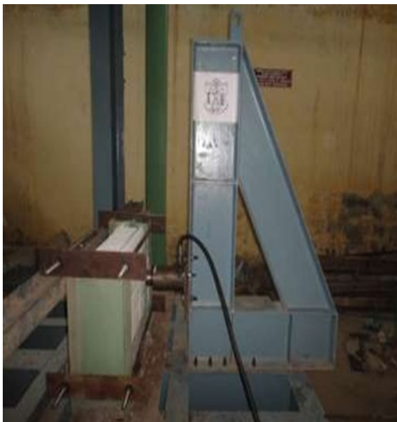
Fig. 3 Out-of-plane testing on GPC wall
