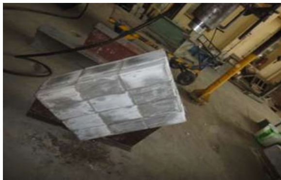
Fig. 1 Set up for diagonal compression test
