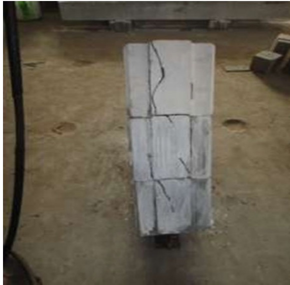
Fig. 2 Crack pattern due to diagonal compression test
