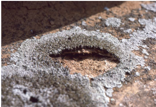
Fig. 9.3 Section through Lecanora muralis to show the blister created on the shoulder of a terracotta pot at the Museo Nazionale Romano—not only has pottery been detached from the surface to a depth of 2–4 mm, but a chamber to a depth of 3–5 mm beneath this has created a microenvironment which influences other biodeterioration processes (Seaward 1988)
