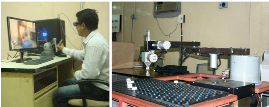
Fig. 3.2 Left A 6-DOF Phantom™ being used for manipulating a 6-DOF manipulator. Right A 3-DOF planar manipulator
