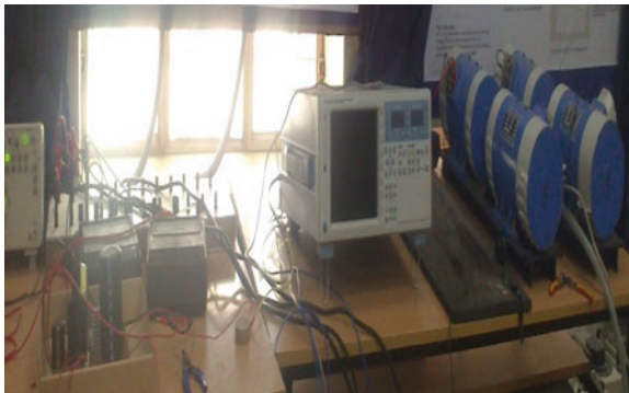
Fig. 13.7 Experimental setup for the measurement of DC power at DC/DC boost converter
