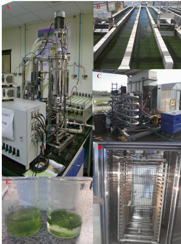
Fig. 2 (a) An R&D type of photobioreactor, (b) concrete raceway pond with a paddle wheel, (c) dissolved air flotation (DAF) tank, (d) culture dryer (industrial scale), (e) flocculated culture
