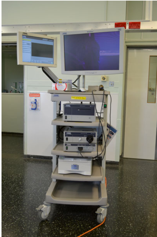
Fig. 7.3 Stack system with High Definition screen, connected to camera and endoscope
