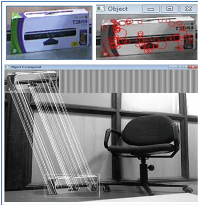
Fig. 2 The image of the target object to be detected (top left); blob features identified on template image (top right); matching of key points of the object from the template image to the corresponding key points of the same object in the image captured by Kinect during navigation (bottom)
