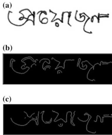
Fig. 4 Fractal dimension-based feature. a Original component. b Upper part of the contour. c Lower part of the contour
