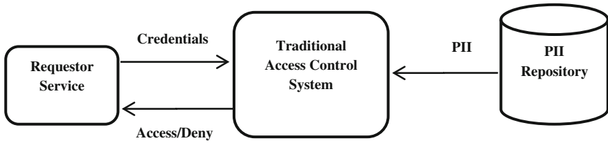
Fig. 1 Traditional access control system
