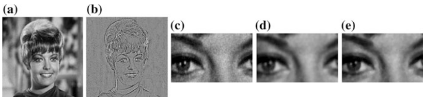
Fig. 4 a Original image. b Sharpened image. c Noisy image. d Gaussian filter. e Median filter
