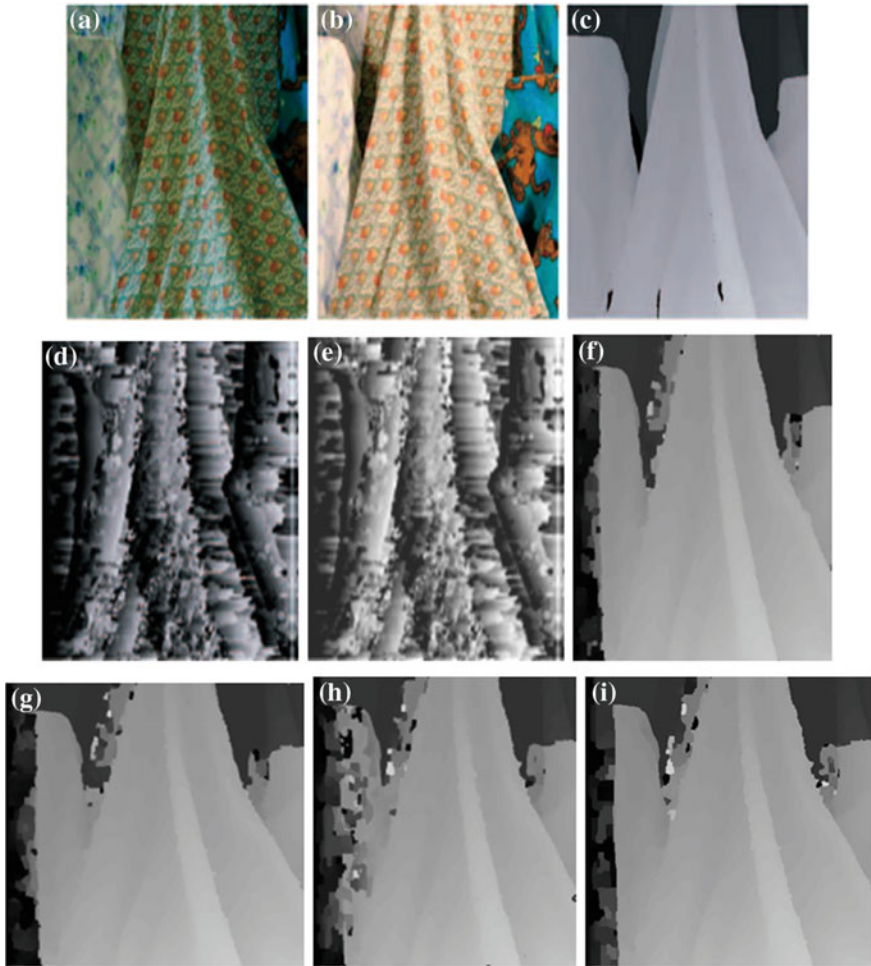
Fig. 4 Results of Cloth stereo algorithms with varying illumination. a Left. b Right. c Ground. d SAD. e SSD. f NCC. g ZSAD. h ZSSD. i ZNCC
