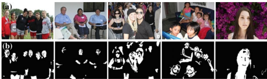
Fig. 6 Sample output of the skin detection stage a original images and b detected skin region in each image
