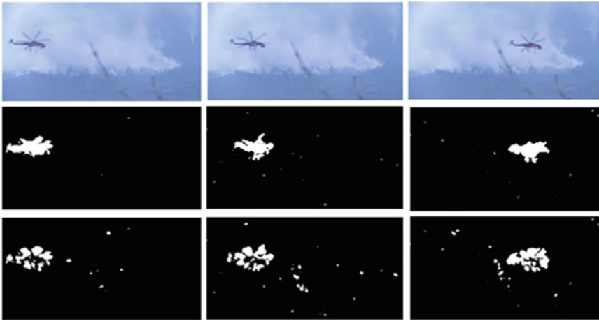
Fig. 4 Comparison of results on helicopter sequence. The top row is the original 51269th, 51276th and 51316th frames. The second row is the results obtained by our proposed method, and the results obtained by Xue et al. [1] method is shown in the third row
