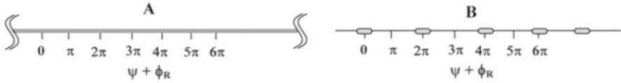
Fig. 7.3 Bunching of electrons by the ponderomotive wave. “A” shows an un-bunched electron beam with uniform distribution of electrons (gray) over all phases of the ponderomotive wave and “B” shows electrons bunched around phases 0, \pi, 2\pi , etc.
