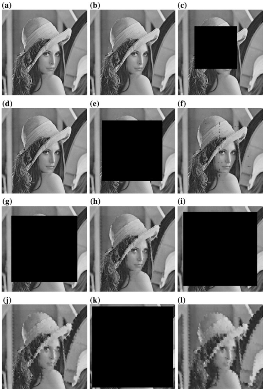
Fig. 12 a Original Lena image; b watermarked image of (a) with PSNR = 41.44 and SSIM = 0.93; c image in (b) tampered by 25 % cropping at center; d recovered image from (c) with PSNR = 35.51 and SSIM = 0.90; e image in (b) tampered by 50 % cropping at center; f recovered image from (e) with PSNR = 30.91 and SSIM = 0.85; g image in (b) tampered by 60 % cropping at center; h recovered image from (g) with PSNR = 30.07 and SSIM = 0.82; i image in (b) tampered by 75 % cropping at center; j recovered image from (i) with PSNR = 27.55 and SSIM = 0.7645; k image in (b) tampered by 90 % cropping at center and l recovered image from (k) with PSNR = 24.91 and SSIM = 0.67
