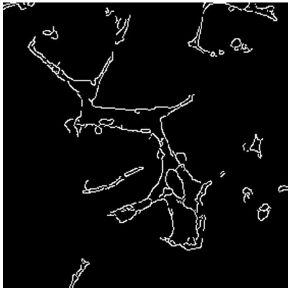
Fig. 19 Image after removal of too short edges
