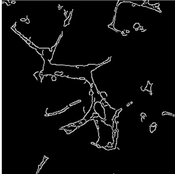
Fig. 18 Image after use of Canny–Deriche edge detector
