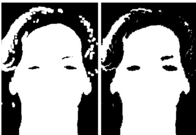
Fig. 15 Face area after erosion on the left , and on the right face area after dilation
