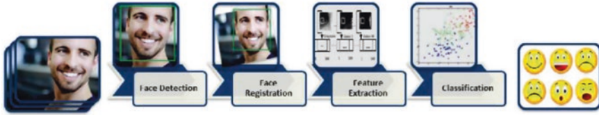
Fig. 8.1 Typical processing pipeline for facial expression analysis
