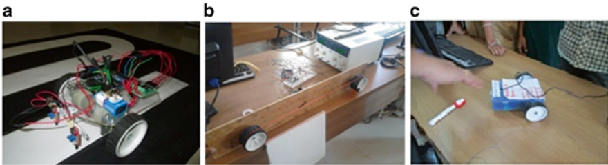
Fig. 2 (a) Line following robot (b) Automatic door open and close (c) Obstacle avoiding robot
