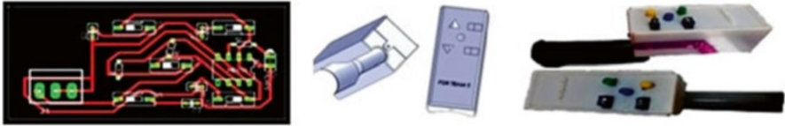
Fig. 1 PCB layout, CAD design and working prototype
