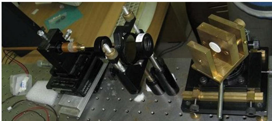
Fig. 8 Angular interrogation setup for SPR experiments [17]
