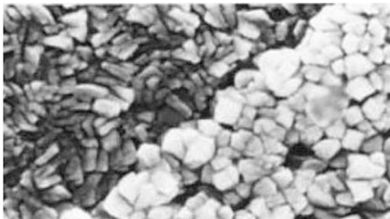
Fig. 6 SEM of a film with simultaneously deposited \alpha - \text{Fe}_2\text{O}_3 and \text{Fe}_3\text{O}_4 , revealing morphology characteristic of differing crystal structure
