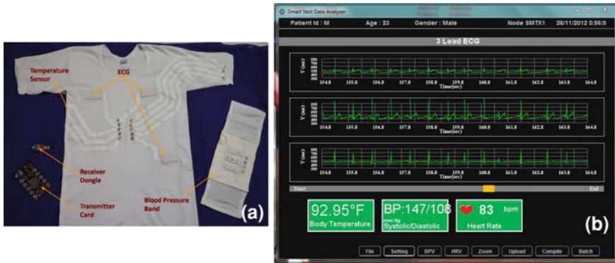
Fig. 8 e-vest with conductive textile electrodes for 3 lead ECG, printed traces to connect sensors and flexible electronics, Photoplethysmography band for Pulse Transit time based blood pressure estimation, wireless communication through ZigBee and real-time data display [33]
