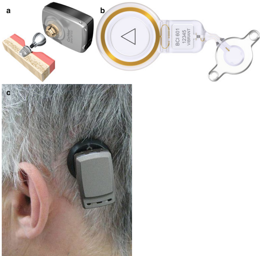
Fig. 2.5 (a) Bone conduction devices – Percutaneous Baha (Courtesy Cochlear Ltd). (b) Bonebridge (Picture Courtesy MED-EL). (c) Bone conduction device – Baha Attract (Courtesy Cochlear Ltd)
