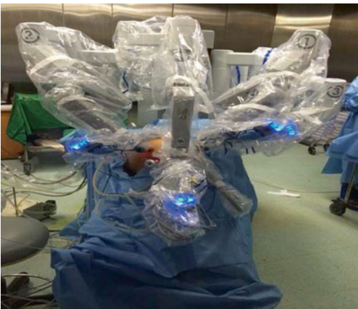
Fig. 21.10 Widely spaced arms after docking between legs
